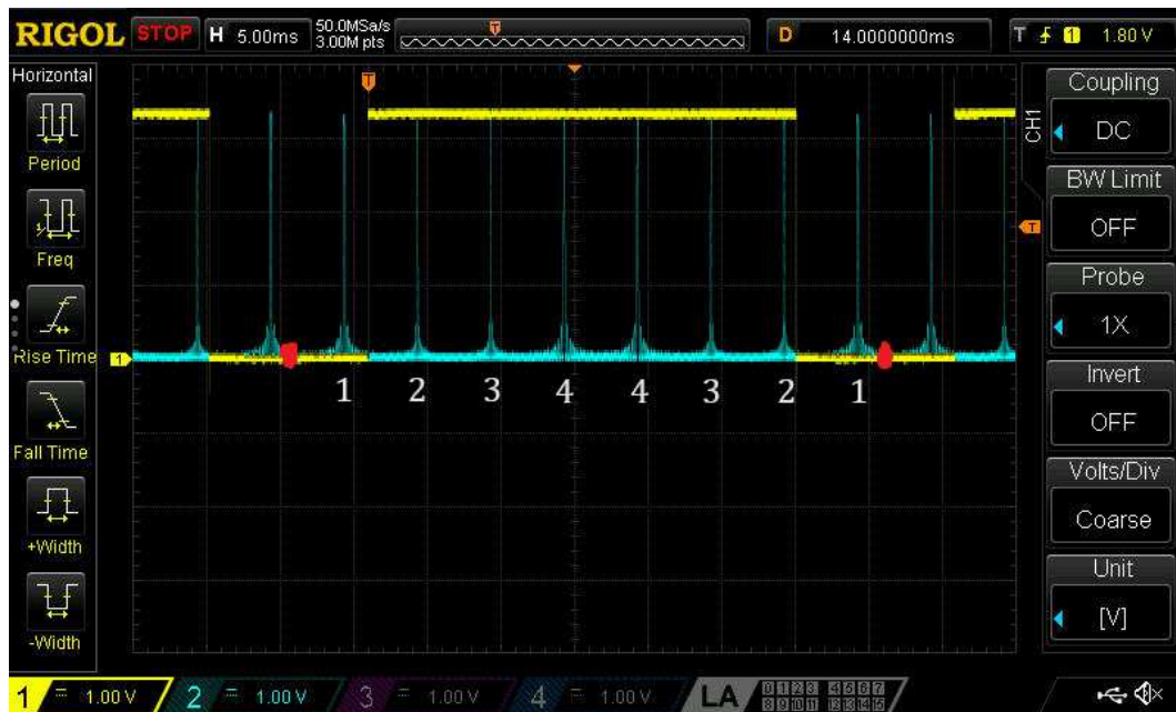
Figure 4.12 – Oscilloscope Emulation Results - Displaying Data from All Four FBGs.
