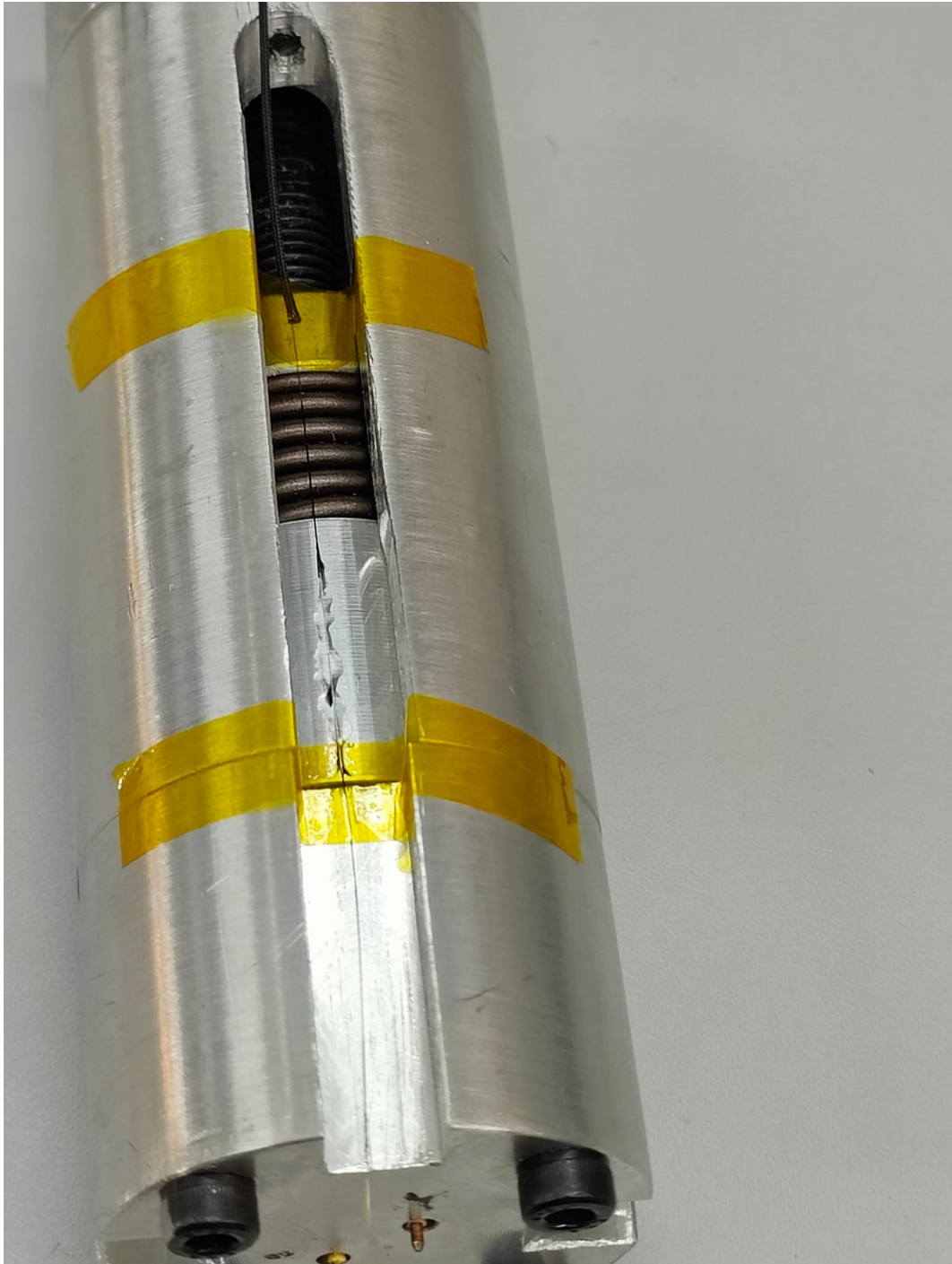
Figure C.1 – First extremity bonded and fixed with Kapton tape.
