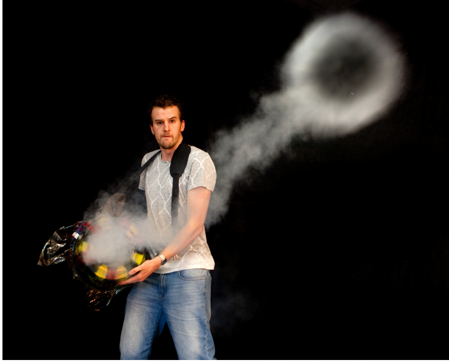
Figure 1.3: Experiment showing the formation of a smoke ring. The smoke is initially undisturbed inside the plastic container. When it's pushed with high velocity against the round opening, the smoke takes the form of a ring [23].
