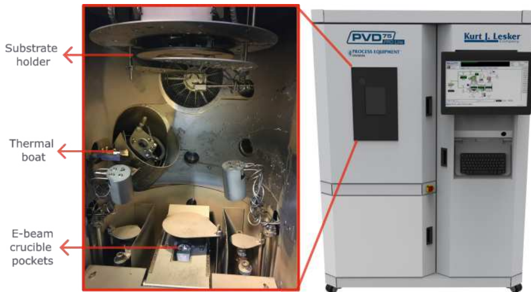
Figure 2.5: PVD75 equipment from Kurt J. Lesker company, used in this work (adapted from [49]).
