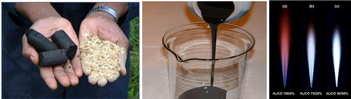
Figure 3.7. Fast pyrolysis products: biochar (left, with biomass to its right) (Hamilton, 2007), bio-oil (center) (Iowa State University) and syngas burning flames (right) (Hwang et al. , 2013)
