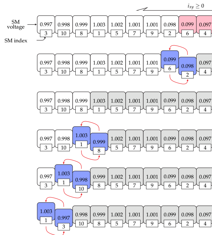
Figure 8. Submodule voltage sorting process.
