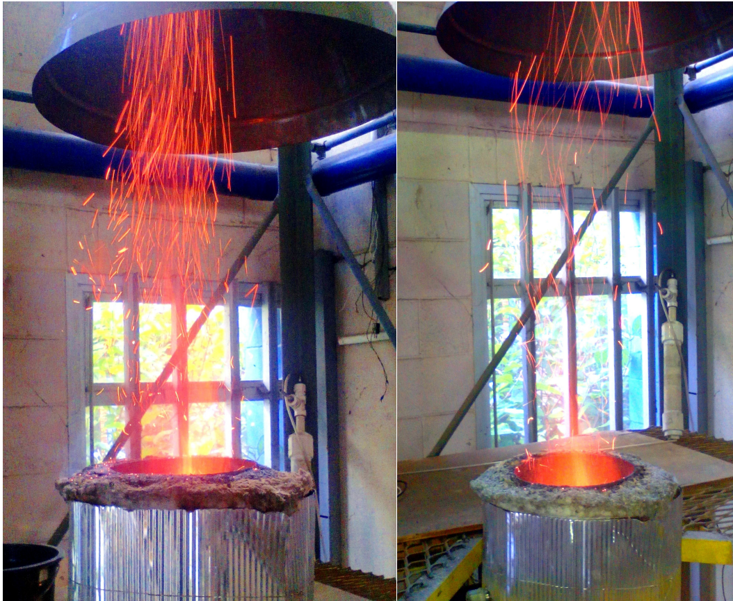
Figure 4.2 – Images from the reactor top during experiments of sugar cane leaves and bagasse mixture. The left and right photographs were taken along the sample's combustion steady state phase and residual char combustion phases, respectively.
