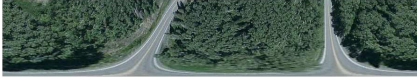
(c) Aerial image shown in Figure 2.2(a) after polar coordinates transformation.
