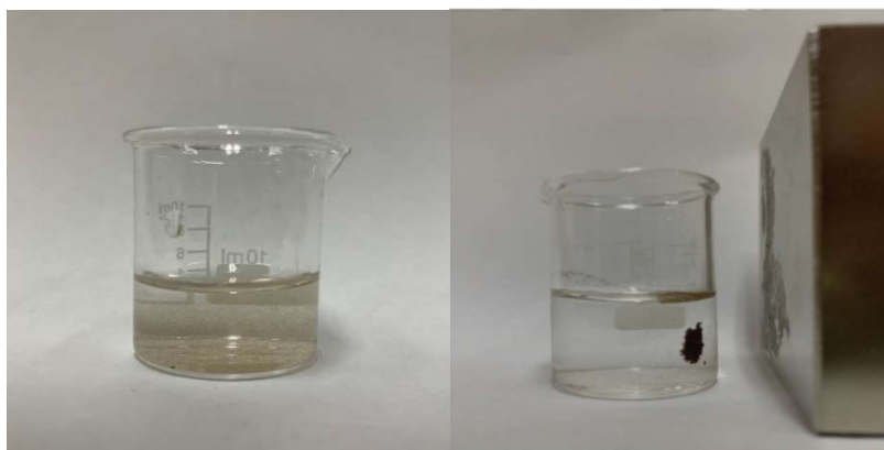
Figure 3.7 – GO/mCS/OC separation with magnet.
