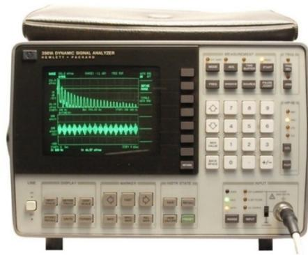
Figure 7-1 Agilent HP 3561A Dynamic Signal Analyzer
