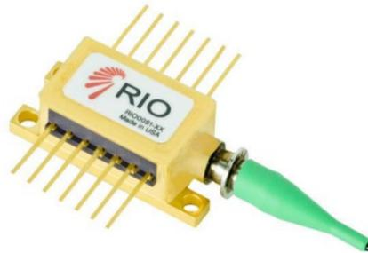
Figure 7-2 RIO PLANEX™ Series 1550nm Low Phase Noise Narrow Linewidth External Cavity Laser
