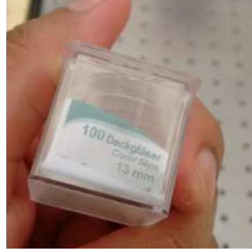
Figura 3.6 – Borosilicate glass substrate used for gold deposition.
