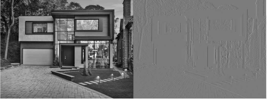
Figure 3.5 – Vertical Edge Detector Example: In this image, a simple hand-designed convolutional kernel was employed to detect vertical edges across the entire image. Image inspired in (GOODFELLOW et al. , 2016).
