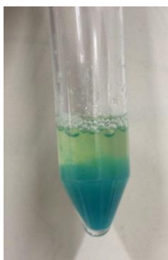
Figure 3 - Sample precipitation following the Folin antioxidant test.
