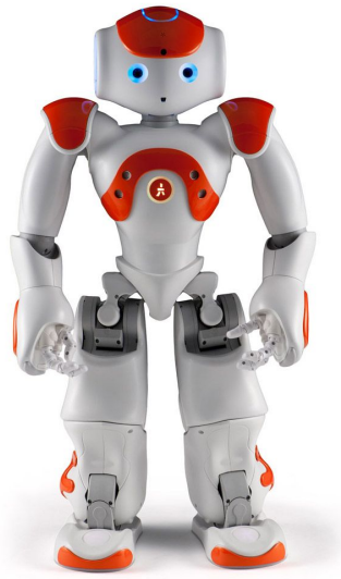
Figure 4.1: An overview of the NAO humanoid robot. It showcases highly articulated limbs and torso, enabling natural interaction and movement emulation. Equipped with a range of sensors, NAO is a versatile platform for research in human-robot interaction and cognitive robotics.
