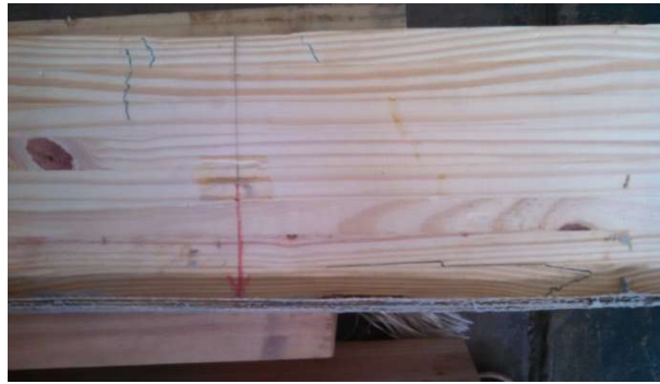
Figure 17. Detail of the compressive rupture of the Vectran fibers reinforced beam.
