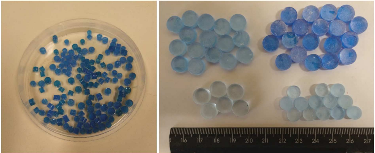
Figure 3.11 – Manufactured particles with different diameter after curing process. Note that particles on the right are covered in talcum powder to avoid sticking and present different colors according to the amount of pigment added in the polyurethane mixture before degassing.
