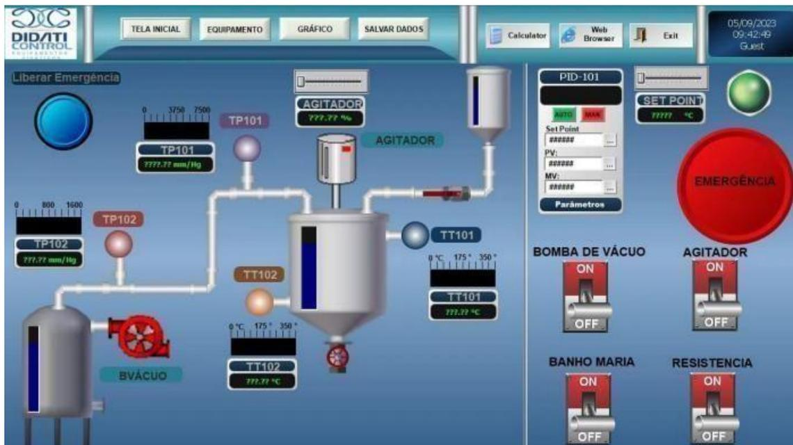
Figure 6.3: Screen control for the pilot plant [Author's source].
