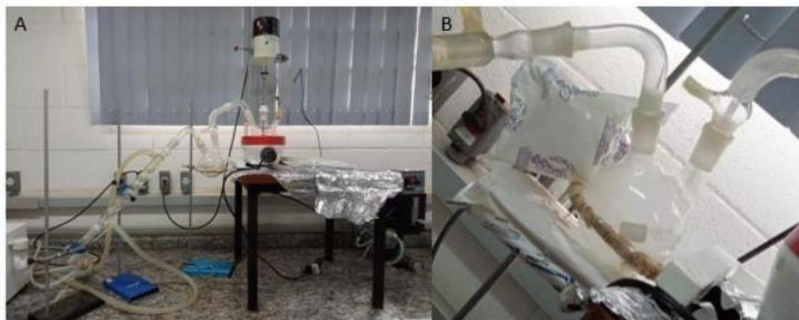
Figure 4.4: The part a) represents the scheme for L-lactide production; The part b) details of the configuration, especially the L-lactide reservoir where the ice was placed [Author's source].
