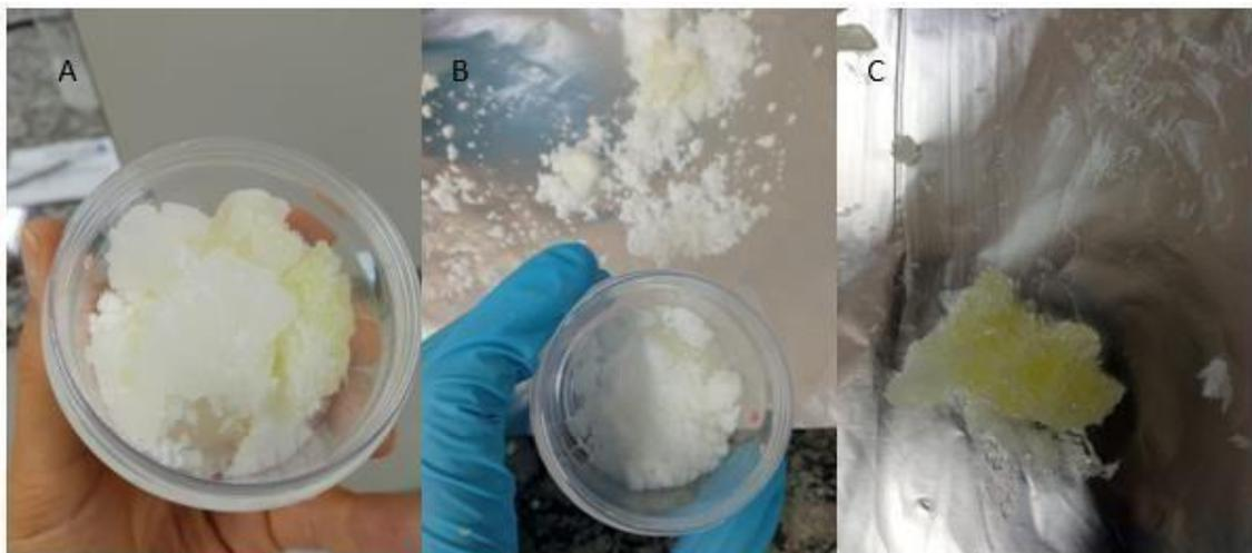
Figure 4.6: The part a) and b) represent the L-lactide produced dry; The part c) represents L-lactide with water. It can be observed the formation of crystals, but it is possible to notice that a part of it is still moist [Author's source].
