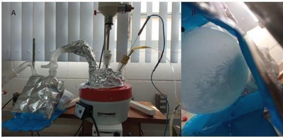
Figure 4.5: The part a) represents the scheme for L-lactide production with aluminium; The part b) represents the details of the production of L-lactide crystals [Author's source].
