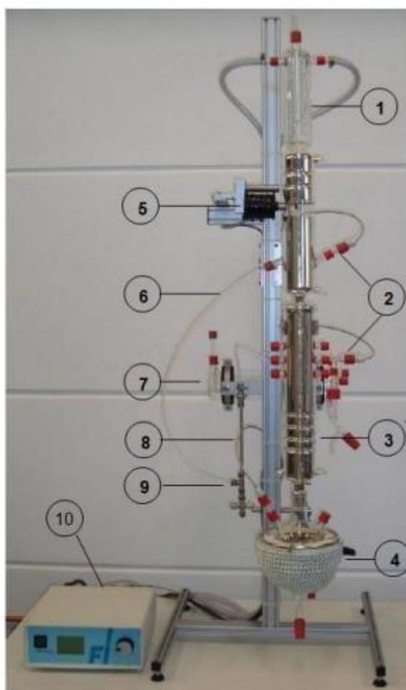
Figure 4.1: Reactive distillation system. (1) condenser, (2) thermocouples, (3) reactive distillation column, (4) reboiler, (5) solenoid valve, (6) recycle, (7) decanter, (8) pre-reactor, (9) mixer, (10) controller [Author's source].
