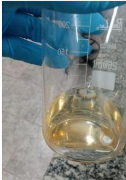
Figure 6.12: L-lactide collected after these two steps of purification [Author's source].
