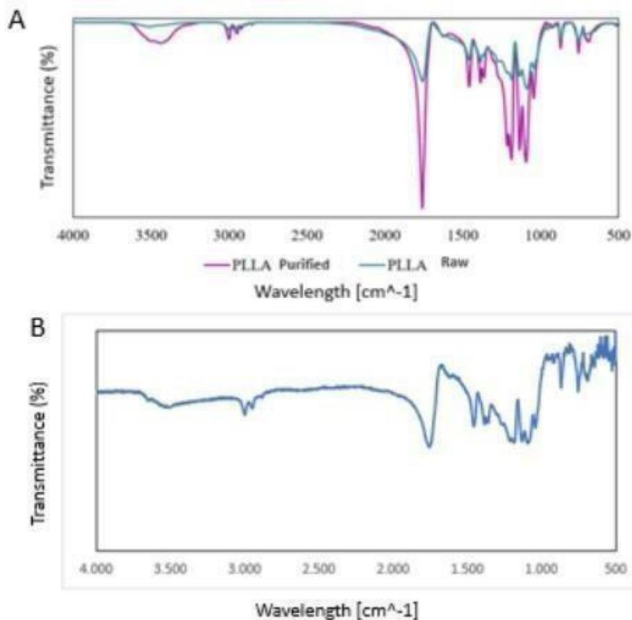
Figure 6.13: the part A showed the FTIR done for the PLLA in the experimental unit and the part B shows the FTIR of PLLA produced in the Pilot Plant [Author's source].
