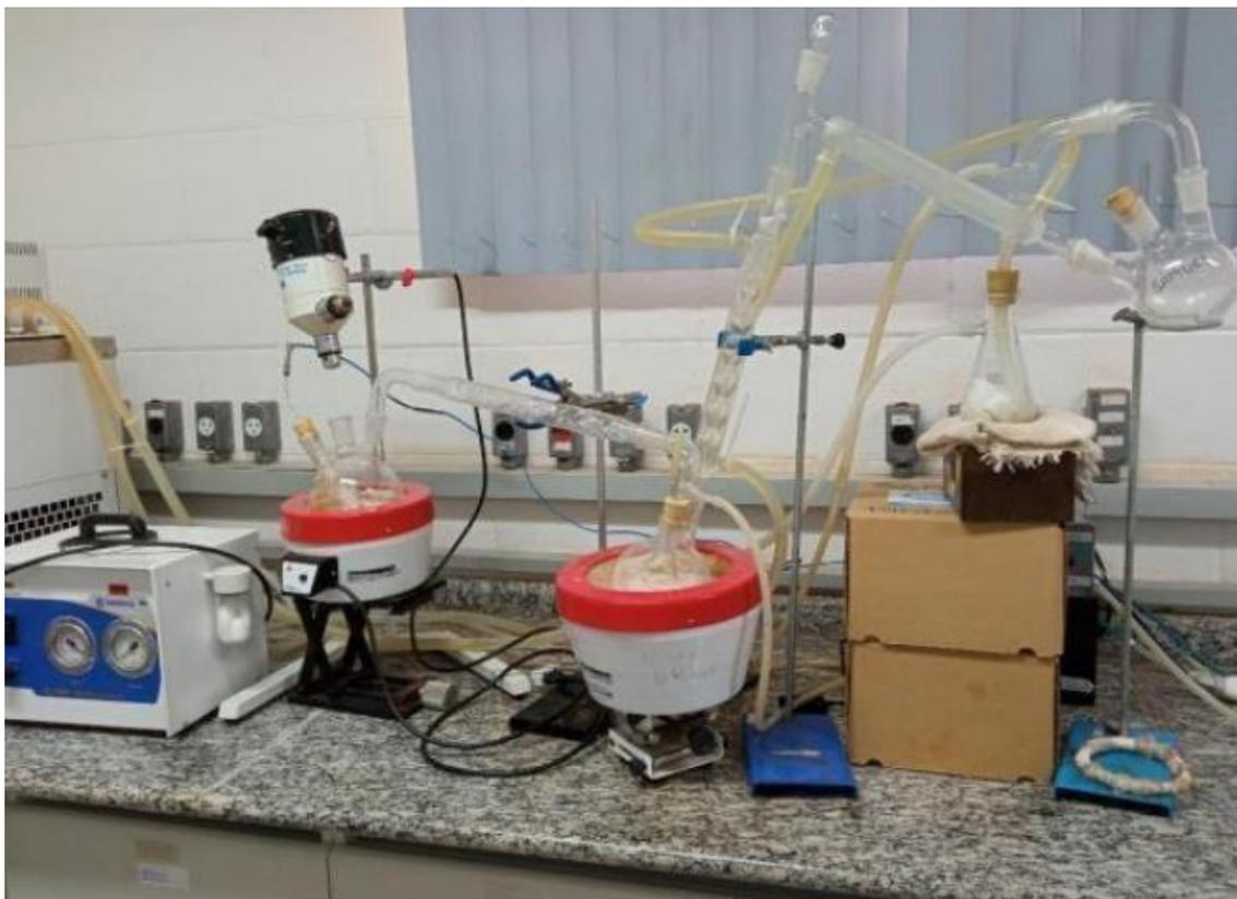
Figure 5.5: The third configuration done for producing PLLA and L-lactide [Author's source].
