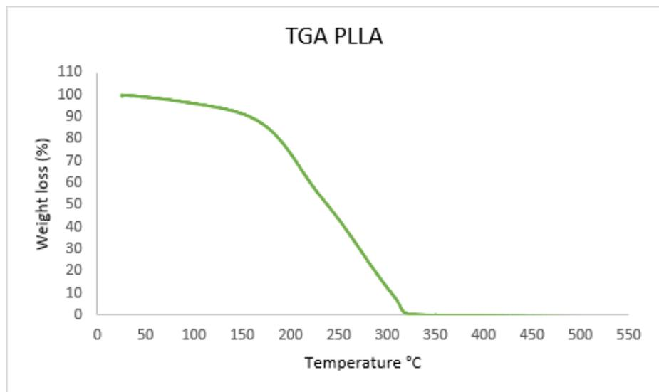
Figure 4.16: TGA curve about PLLA produced [Author's source].
