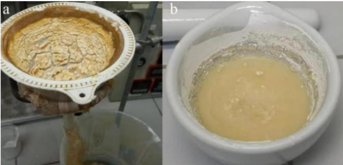
Figure 5.15: Filtered solution (a) and transferred purified PLLA (b) [Author's source].
