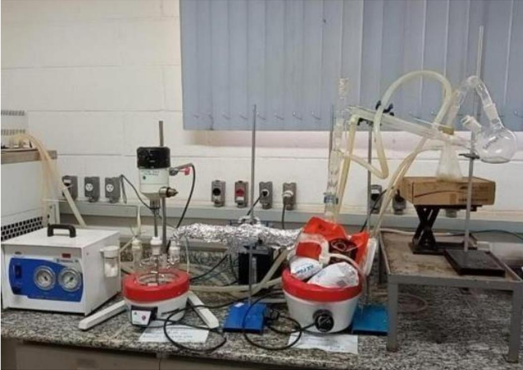
Figure 5.8: The fourth configuration done for producing PLLA and L-lactide [Author's source].
