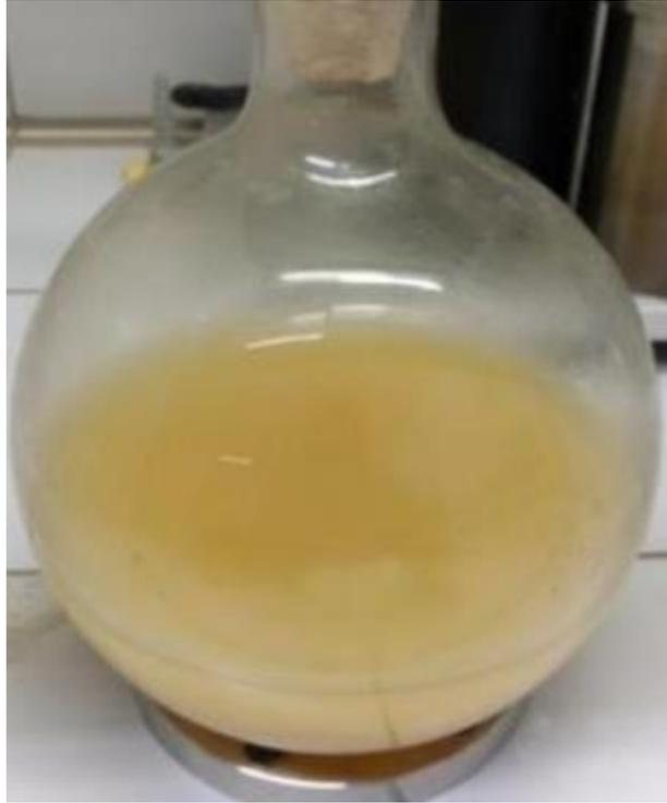
Figure 5.14: Solution with PLLA and chloroform precipitated with ethanol [Author's source].
