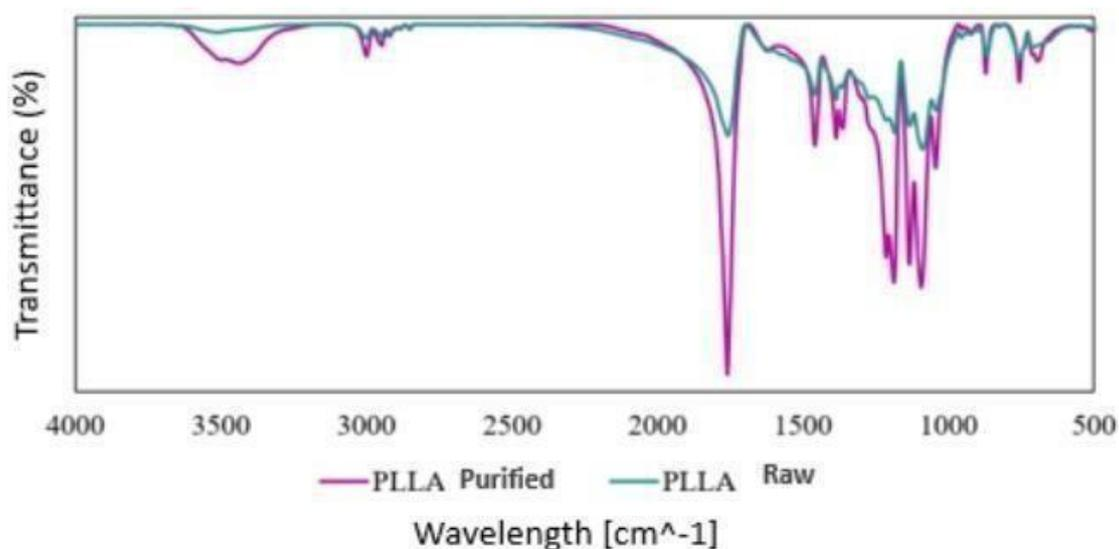
Figure 5.19: FTIR of PLLA obtained from polycondensation in the Fourth configuration before and after the purification process [Author's source].
