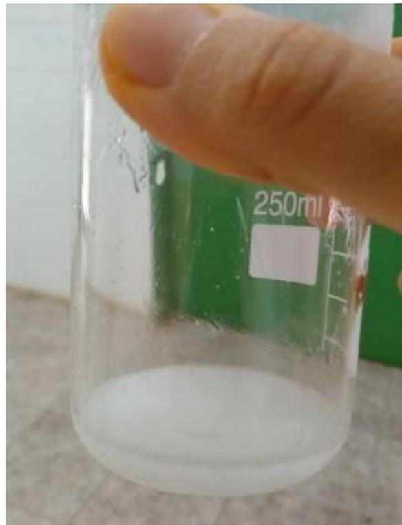
Figure 4.10: PLLA produced from ring-opening route [Author's source].
