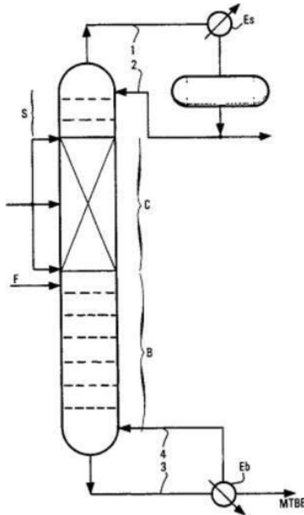
Figure 2.6: The reactive distillation scheme presented by Roi et. al, in the patent number 5,368,691 (ROI et al., 1994).
