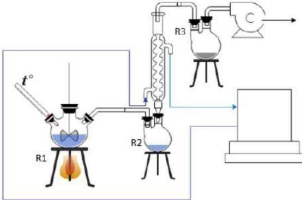
Figure 5.3: Diagram of the system for increased efficiency and conversion of polymer (PLLA) and L-lactide production reaction: R1 represents the reactor of PLLA production, R2 represents L-lactide reserve, and R3 water reserve [Author's source].
