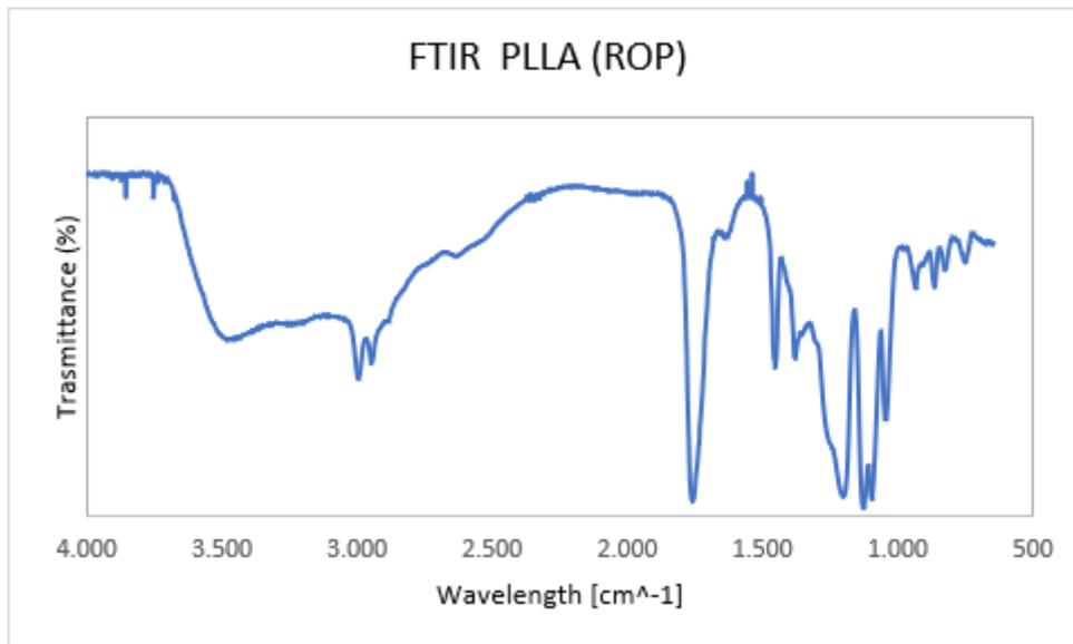
Figure 4.12: FTIR of PLLA produced [Author's source].
