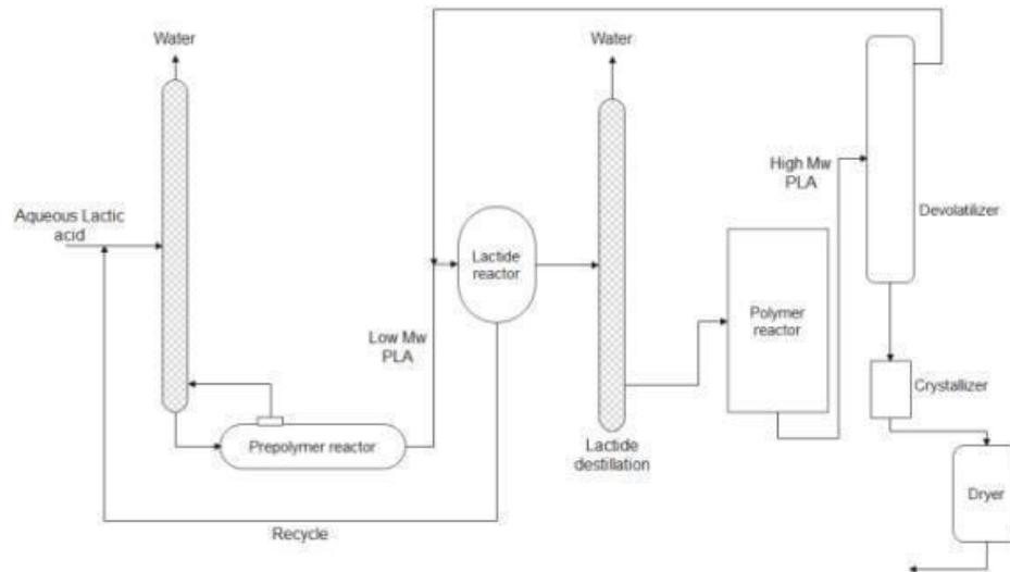
Figure 2.5: The scheme shows the Natureworks™ (Cargill Dow) plant design to produce lactide and PLA (KWAN; HU; LIN, 2018).
