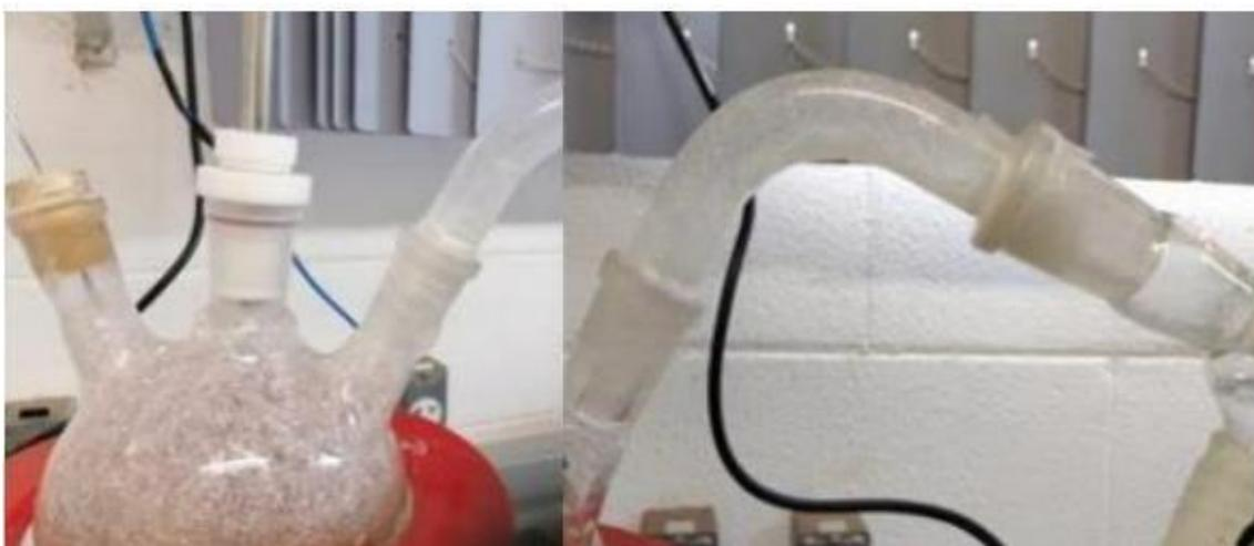
Figure 5.2: Encrustation obtained in 12 h and 8 h respectively (CRIVELLIN et al., 2022a).
