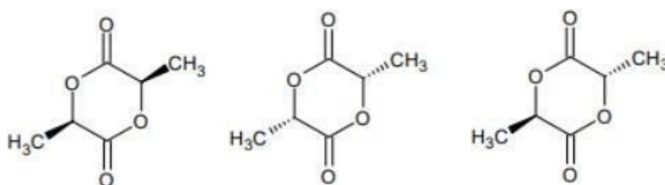
Figure 2.1: Chemical structure respectively of L-lactide, D-lactide, D, L-lactide, Source: Produced in ChemSketch based on (GROOT et al., 2010a).
