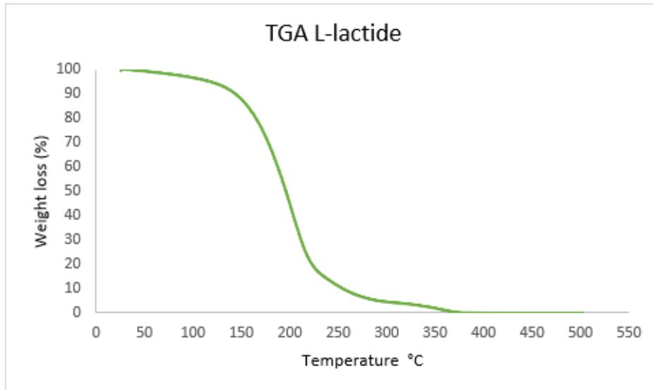
Figure 4.15: TGA curve about cyclic dimer (LLT) produced [Author's source].
