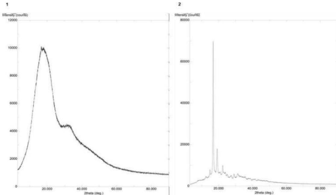
Figure 5.21: XRD of crude (1) and purified PLLA (2) [Author's source].
