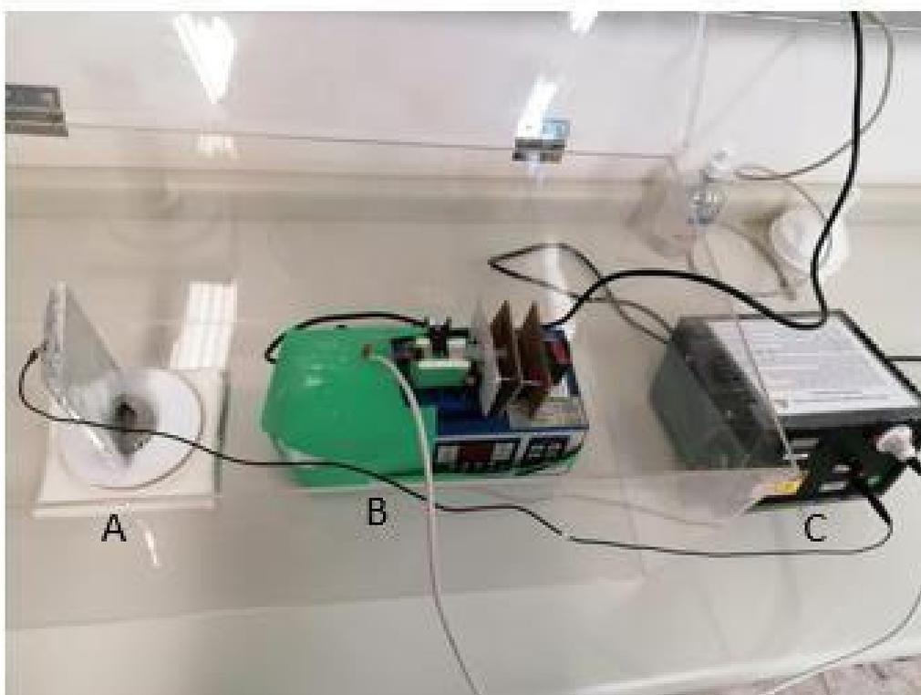
Figure 4.11: Electrospinning equipment parts: A) collector with aluminium part; B) infusion bomb C) High voltage source [Author's source].
