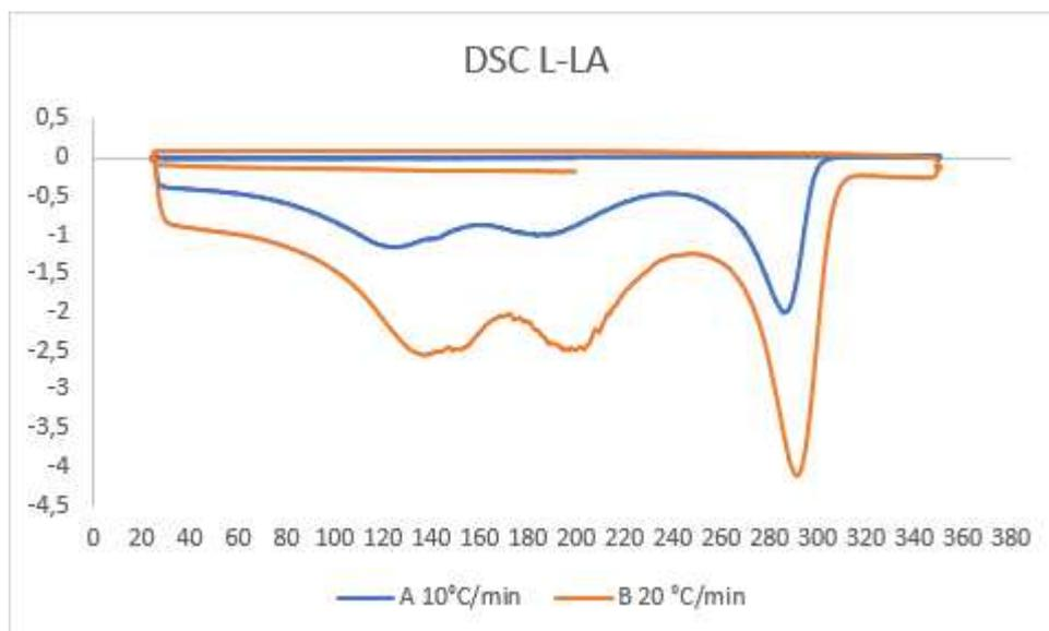
Figure 3.3: DSC analysis for the synthesis of L-lactide [Author's source].
