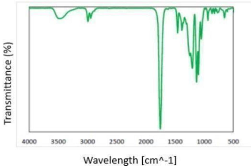
Figure 5.20: FTIR of LLT produced in the Fourth configuration [Author's source].
