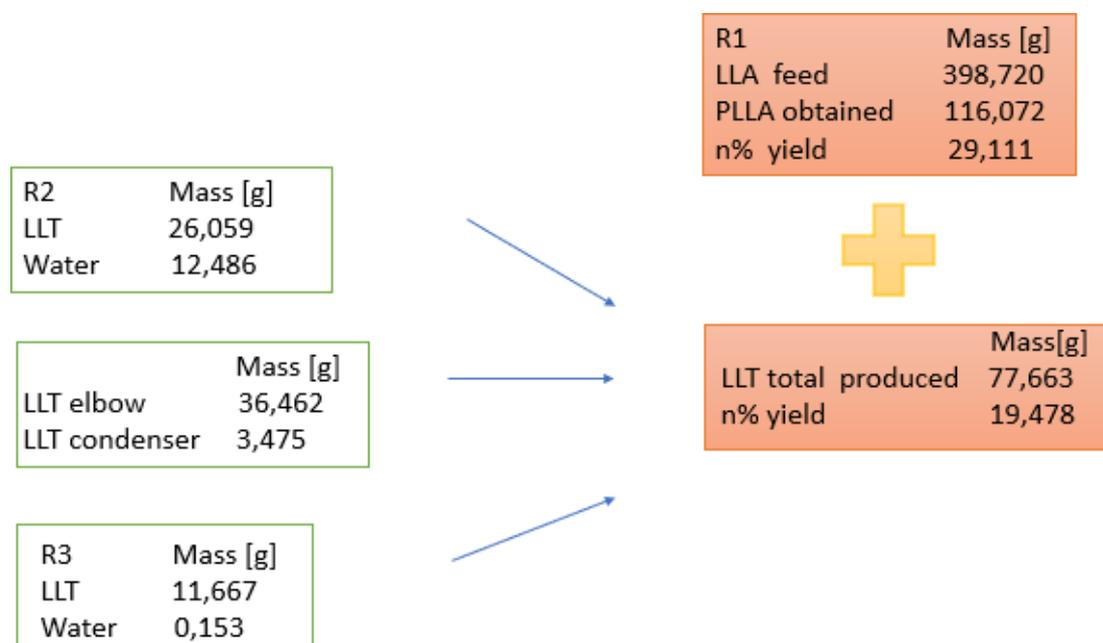
Figure 5.18: Scheme of Mass balance for the Fourth configuration [Author's source].
