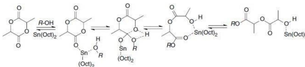
Figure 2.8: General mechanism of PLA chain growth by ROP (HENTON et al., 2005).
