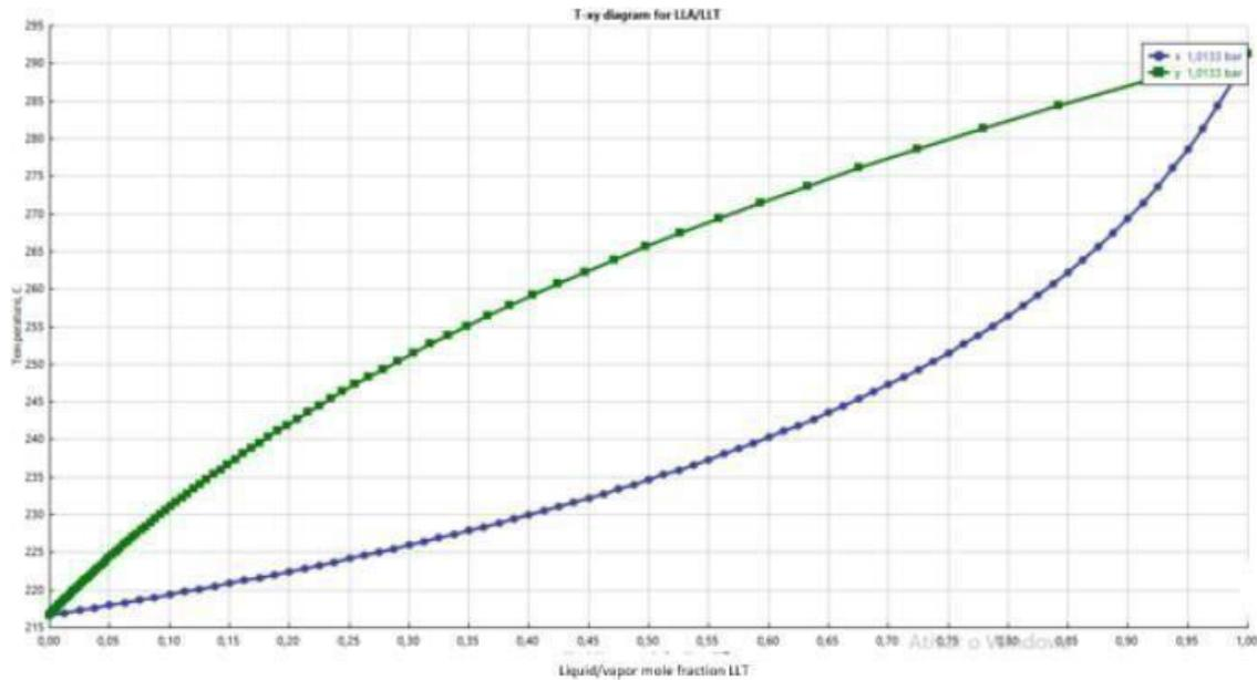
Figure 3.1: Binary mixture liquid/vapor mole fraction with the LLT vary VS temperature [Author's source].
