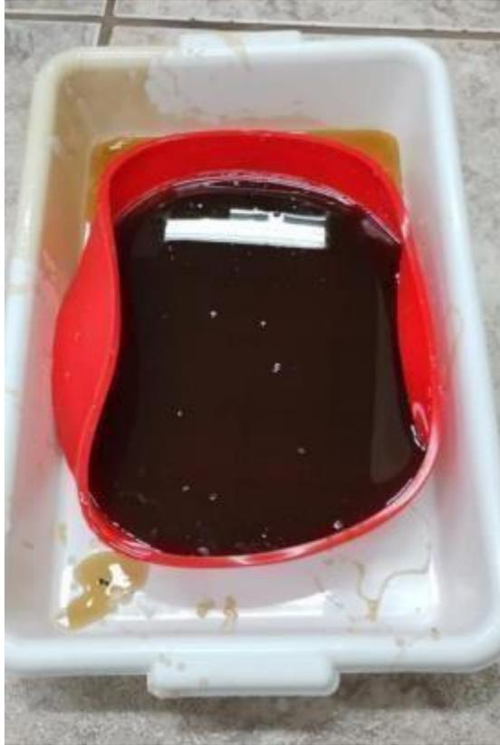
Figure 6.7: PLLA produced in the pilot plant [Author 's source]
