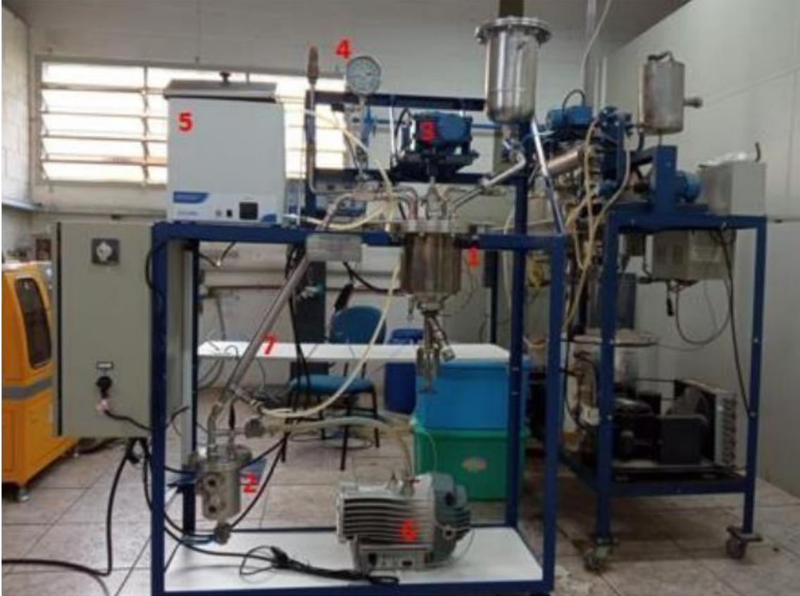
Figure 6.2: Pilot plant for the production of PLLA and LLT [author's source].
