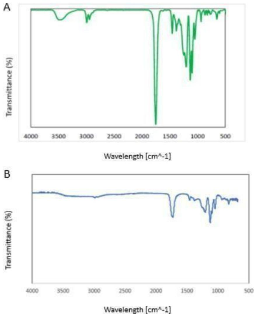
Figure 6.14: the part A showed the FTIR done for the LLT in the experimental unit and the part B shows the LLT of PLLA produced in the Pilot Plant [Author's source].
