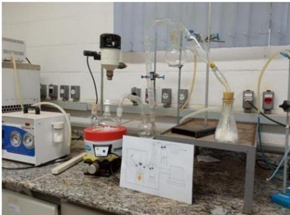
Figure 5.4: The second configuration done for producing PLLA and L-lactide. [Author's source].
