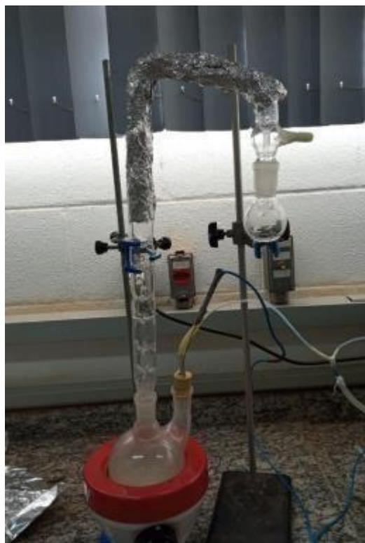
Figure 6.11: Distillation column for the purification of l-lactide [Author's source].
