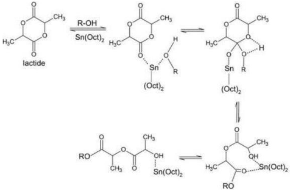
Figure 4.8: Reaction mechanism of the polymerization of PLLA starting from the cyclic dimer LT (CUNHA et al., 2022).
