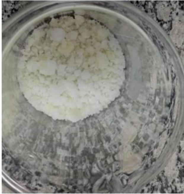
Figure 4.7: L-lactide produced after lyophilization process [Author's source].
