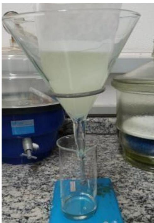
Figure 6.10: Filtration of l-lactide collected in the pilot plant [Author's source].
