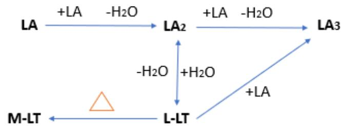
Figure 2.2: Pathways for synthesize LT adapted(PARK et al., 2018).
