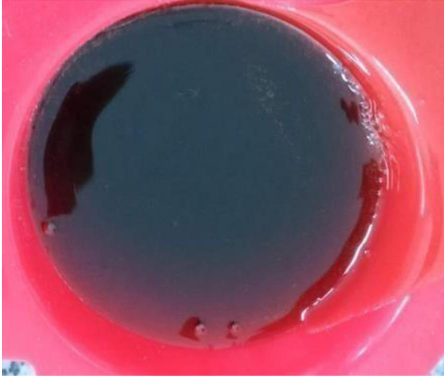
Figure 5.10: Raw PLLA obtained in all configurations [Author's source].
