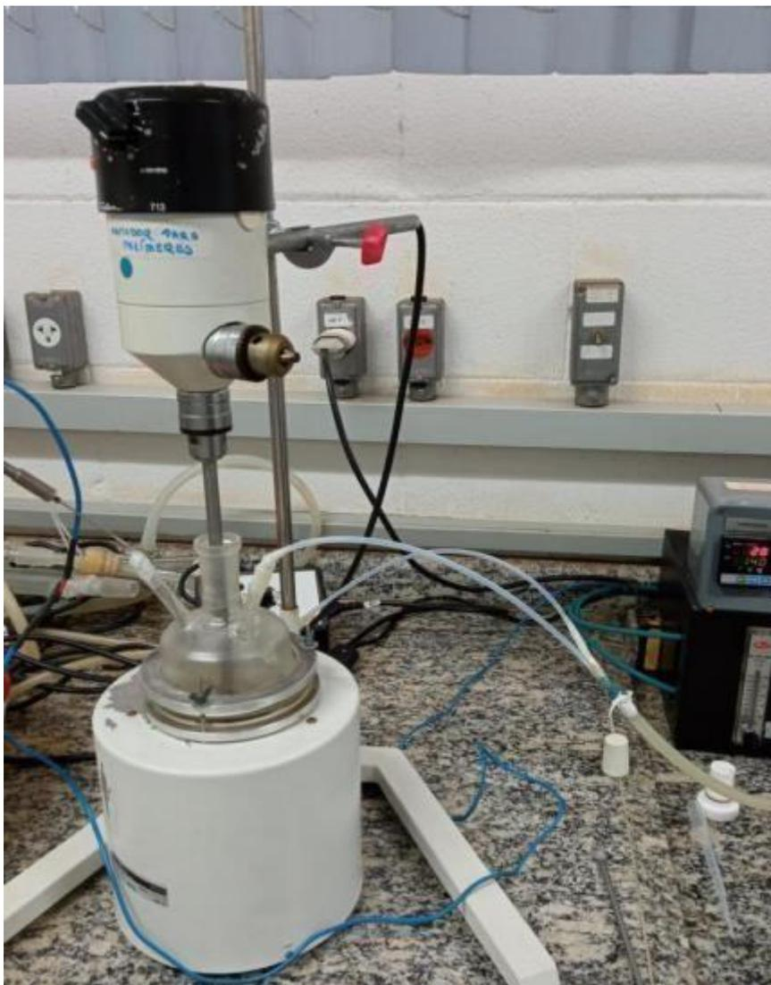
Figure 4.9: System for PLLA synthesis via ROP route [Author's source].
