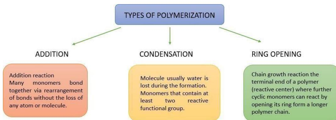
Figure 2.9: Definition on different polymerization techniques (BALAJI et al., 2017).
