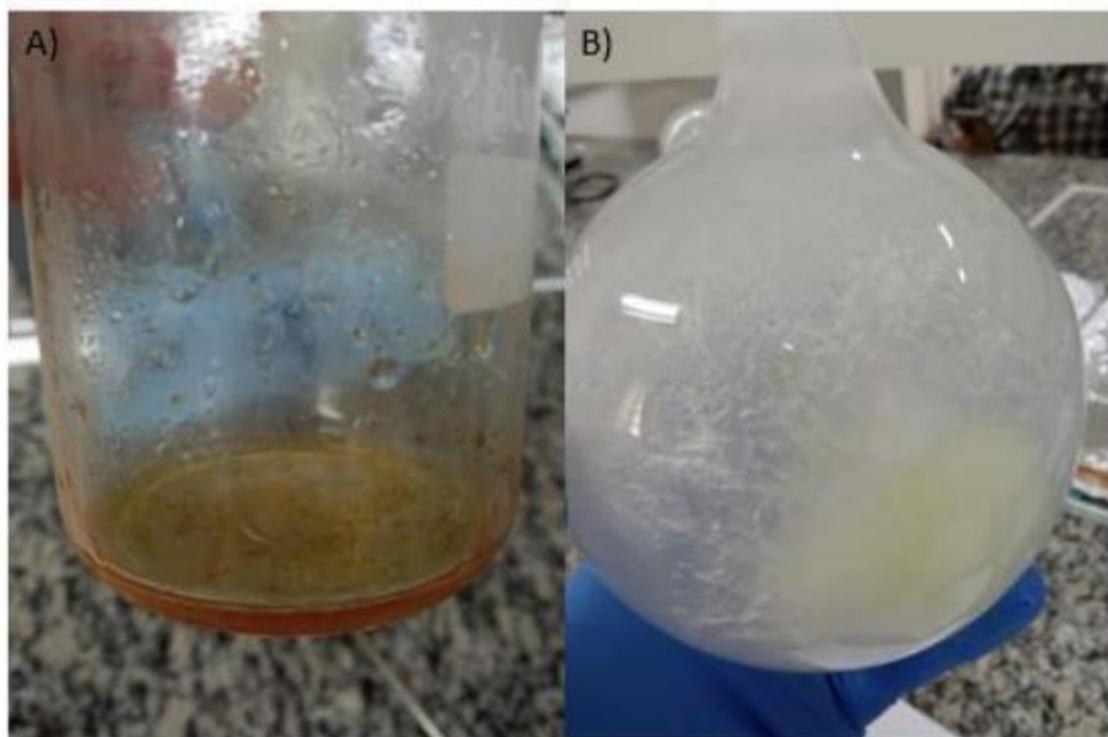
Figure 4.3: The part a) represents the L-lactide produced with N<sub>2</sub> and the part b) represent the L-lactide produced without N<sub>2</sub> [Author's source].
