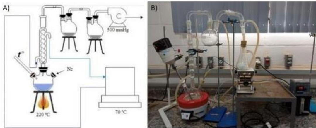
Figure 4.2: the part a) represents the scheme done introducing o N<sub>2</sub> and, the part b) represents the scheme with glass experimental units without N<sub>2</sub> [Author's source].
