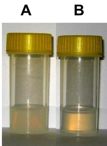
Figure 2.5- Supernatant obtained from milk unsonicated (A) and sonicated at 20 kHz for 60 min (B) (Shanmugam et al., 2012).
