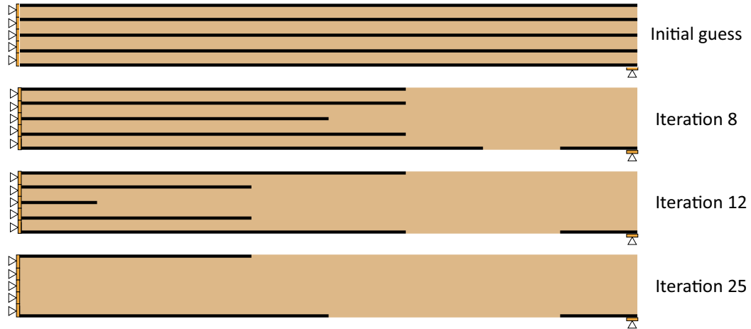
Figure 5.3: Four intermediate topologies with indication of the steel bars position from numerical example 1.
