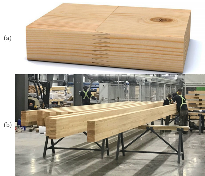
Figure 2.3: (a) Finger joint in a wood piece, image available in https://www.swedishwood.com/wood-facts/about-wood/wood-grades/ (b) GLULAM beam made by Kal Snikoff https://kalesnikoff.com/products/mass-timber-glulam-beams/
