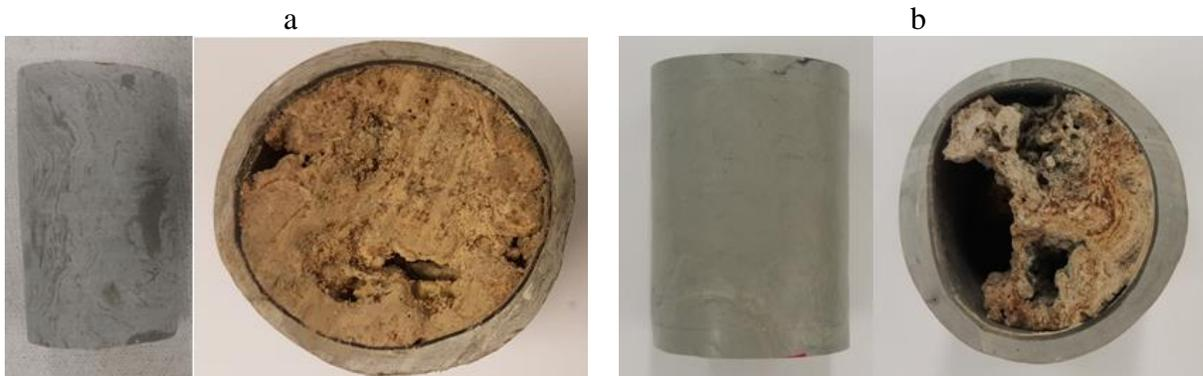
Figure 2-6. a) Third test: applying resin and thermal plastic over the fine-grained plug sample, b) Forth test: applying resin and thermal plastic over the vugular plug sample.
