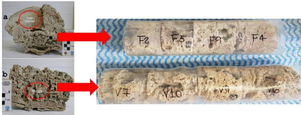
**Figure 1**– Drilled core samples with Workflow of “from block to plug” from microbialite outcrops: a) Fine-grained and b) Columnar facies
