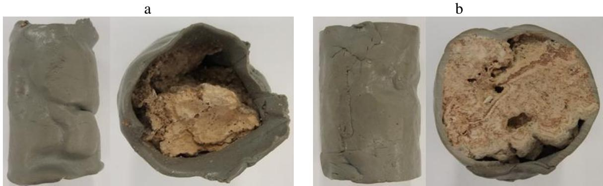
Figure 2-5. a) First test: applying resin directly over the vugular plug sample, b) Second test: applying epoxy resin directly over the fine-grained plug sample.
