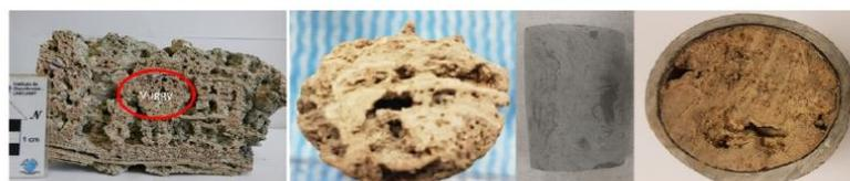
**Figure 1** Samples drilled from columnar/vuggy facies of microbialite outcrops, and prepared for experimental section.
