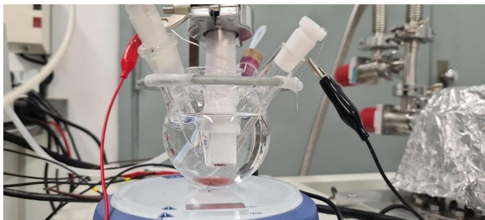
**Figure S2.1.** Custom-made experimental setup for online DEMS measurements during nitrate electroreduction studies. [42]
