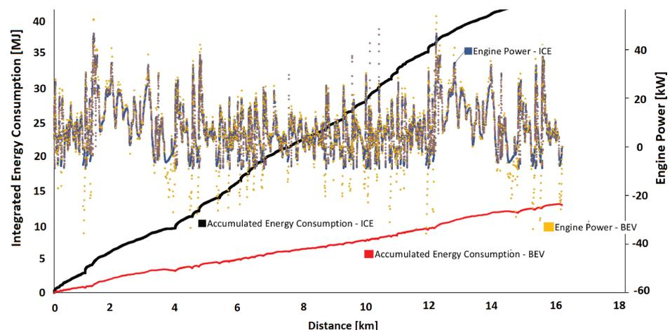
**Figure 4.** Integrated energy consumption for ICEV and BEV during the urban cycle.
