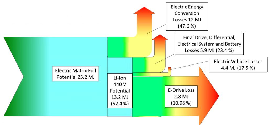
Figure 7. Sankey diagram for the EV model in Highway cycle.
