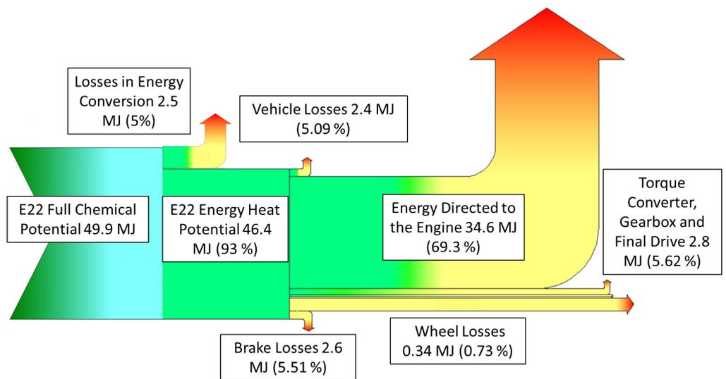
Figure 8. Sankey diagram for the E22 model in FTP 75 cycle.
