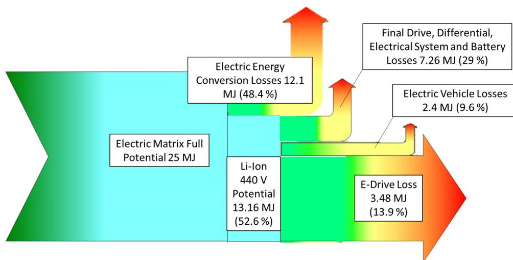
Figure 6. Sankey diagram for the EV model in FTP 75 cycle.
