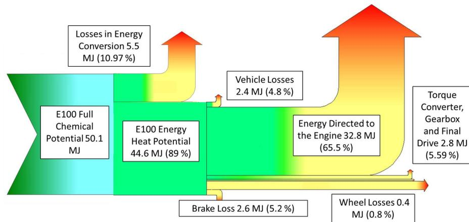
Figure 10. Sankey diagram for the E100 model in FTP 75 cycle.
