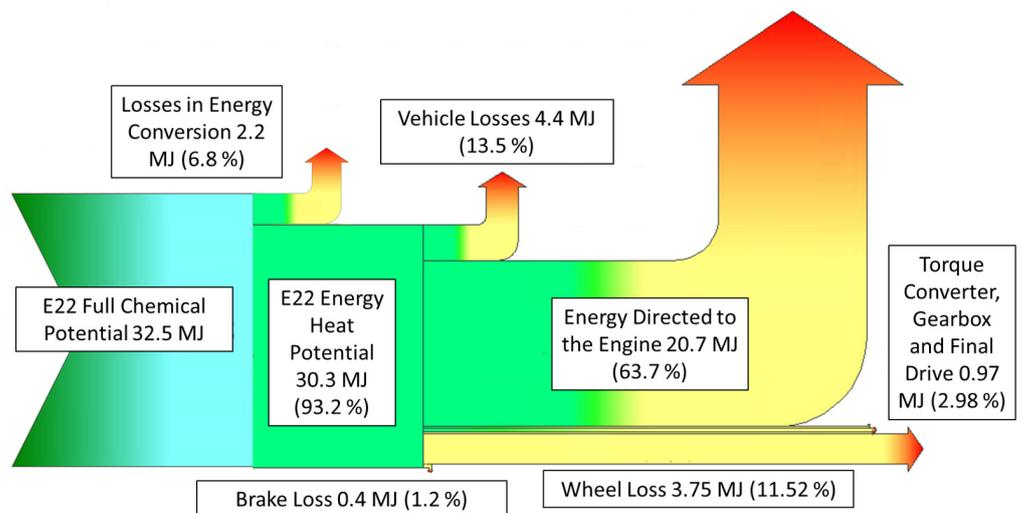
Figure 9. Sankey diagram for the E22 model in Highway cycle.
