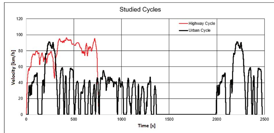
**Figure 3.** Definition of urban and highway cycles based on ABNT NBR 7024. Figure obtained by the authors.
