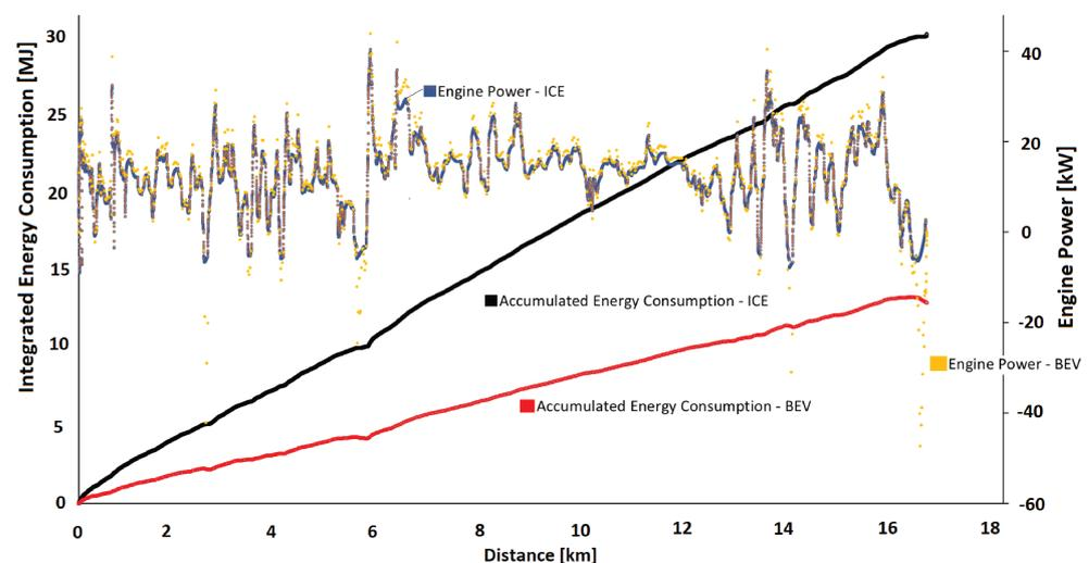
**Figure 5.** Integrated energy consumption for ICEV and BEV during the highway cycle.
