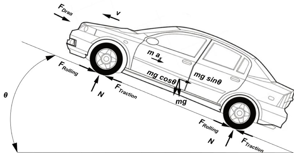
Figure 2. Free body diagram of a moving vehicle during acceleration, obtained in Ref. [5], adapted from [28].
