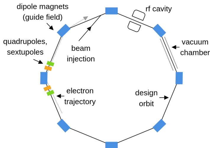
Figure 2: Storage ring typical configuration. Inspired by ref. [11]
