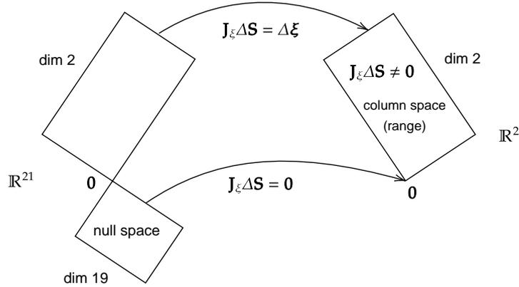
Figure 3.7: Illustration of chromaticity jacobian  $\mathbf{J}_\xi$  fundamental subspaces. The idea is to use sextupole combinations living in the null space, since these are mapped to the zero vector on the chromaticity space.
