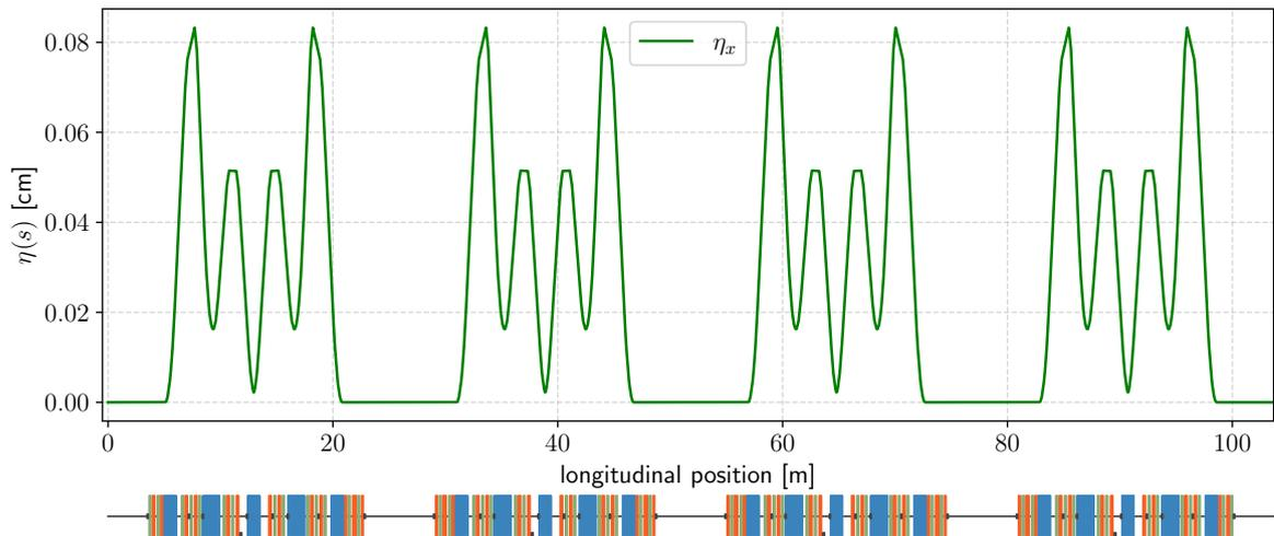
Figure 1.6: Dispersion function for a SIRIUS superperiod.
