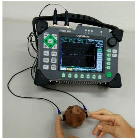
**Figure 5.** Ultrasound test on polyhedra for wood characterization.
