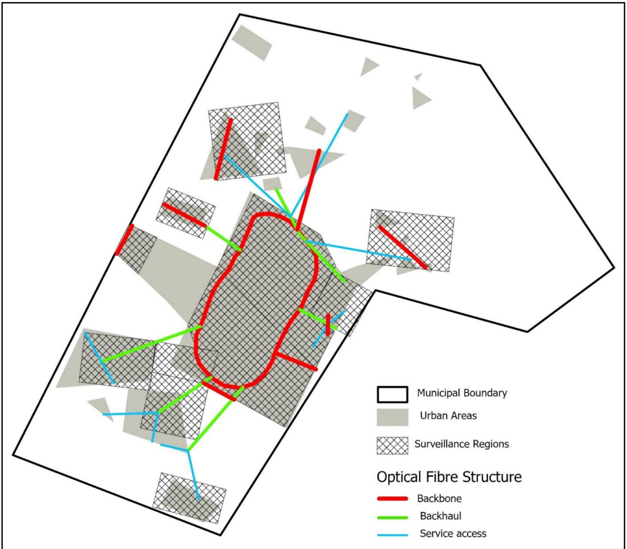
Figure 33 - Optical Fibre and Surveillance structure in Campinas
