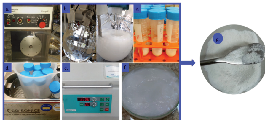
Figure 6. Graphical summary of the synthesis procedure of calcium-polyphosphate (CaPP) particles employing the coprecipitation method: (a) flow pump; (b) controlled addition of CaCl 2 ·2H 2 O solution (1 mL/min; pH = 10) into the NaPP solution; (c) After 4 h of stirring, distribution of the crude product in falcon tubes; (d) washing of CaPP (twice with water and twice with ethanol); (e) Centrifugation after every wash; (f) CaPP slurry obtained; (g) CaPP dried fine powder.
