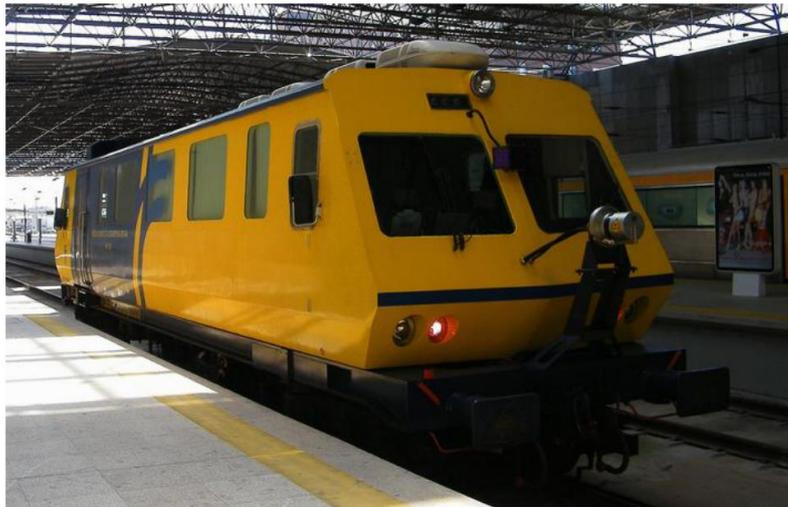
Figure 4: Track geometry car EM 120 - (BERAWI, 2013).
