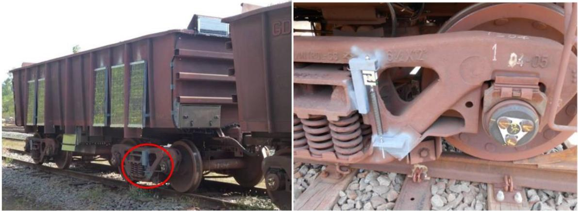
Figure 8: Example of an instrumented railway vehicle (IRV) used in a Brazilian railway. The left figure shows some of the IRVs instrumentation such as solar panels along the carbody. The right figure highlights one of its sensors (load cell attached to spring) for measuring spring displacement – modified from (SANTOS; REICHL, 2014).
