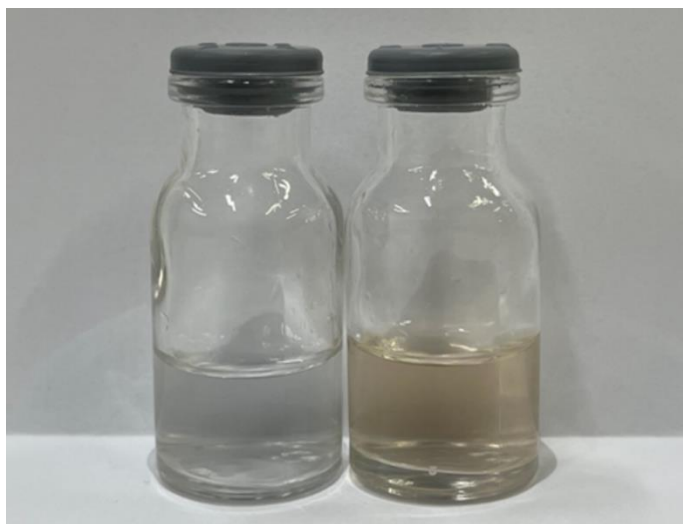
Figure 9. [\text{Fe}(\text{CN})_6]^{4-} solutions with phen before (left) and after (right) the exposure to the UV-Light.
