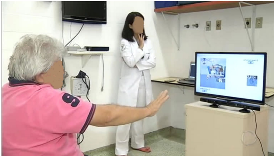
FIGURE 2 Experimental setup: the patient plays GesturePuzzle seated in front to the screen which reproduces the game. Below the screen, a Kinect captures the user movements.
