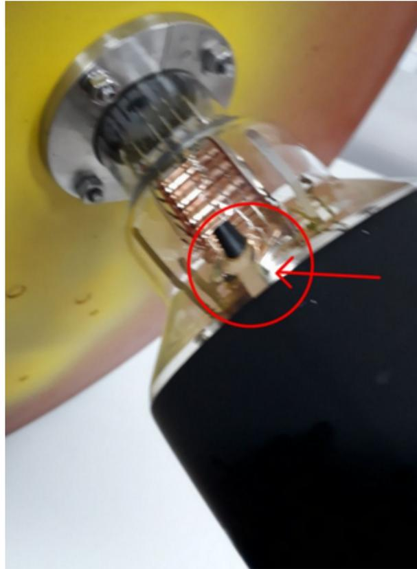
Figure 108 – Conductive material on PMT
