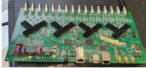
Figure 44 – DAPHNE Front End Board
