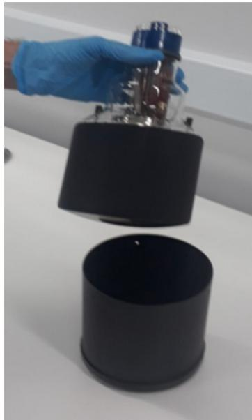
Figure 105 – PMT used in the setup
