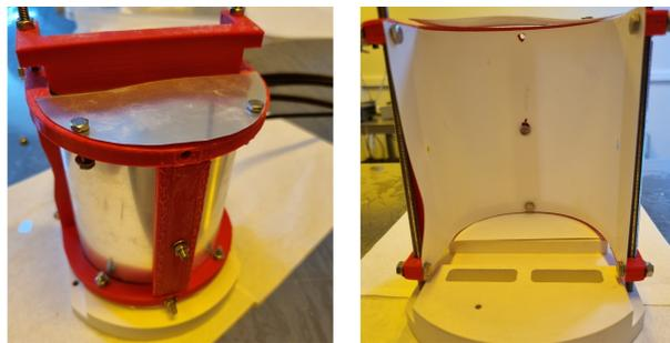
Figure 63 – Support for the X-ARAPUCA and VIKUITI with TPB embedded
