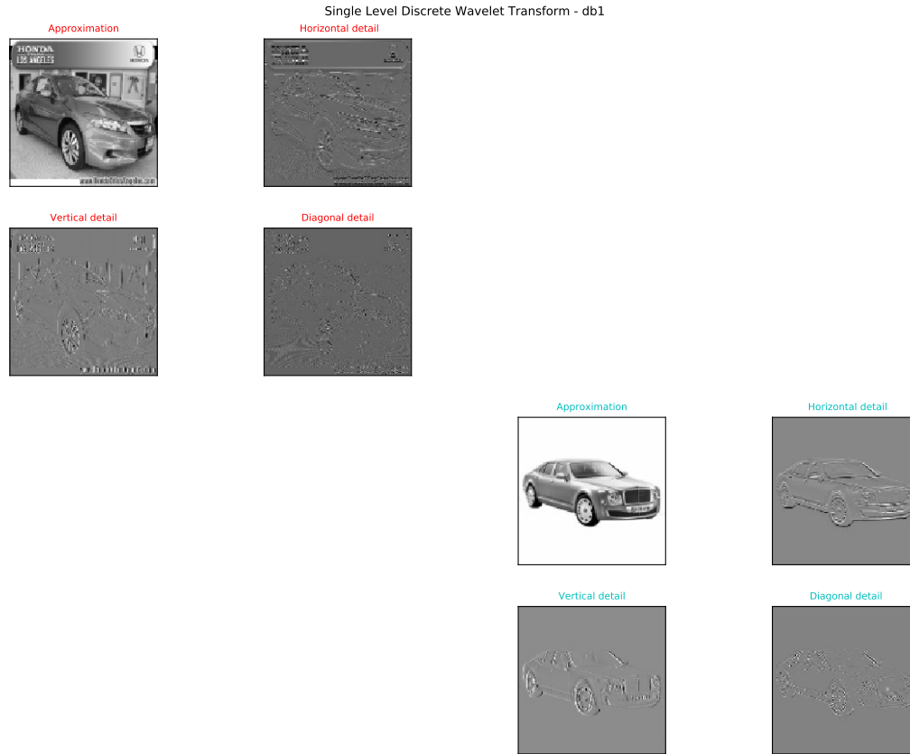
Figure 4.3 – Illustration of single level discrete wavelet transform.
