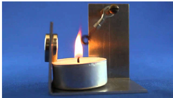
Figure 2.2: Nickel ring reaching its Curie Point and giving in to gravity. Adapted from [10]
