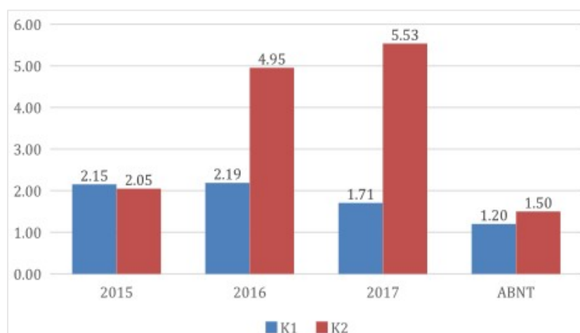
Figure 1 - Comparison between values calculated for the peak coefficients K_1 and K_2 and those suggested by the NBR 12218/2017 (Santos, 2018)
