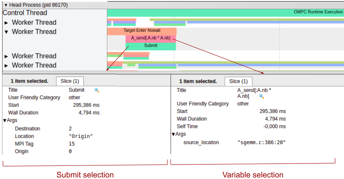
Figure 4.9: Profile symbol usage. The variable event is the one named as A_send[:A.nb * A.nb] , which represents an A_send array of A.nb * A.nb dimensions, and the related nested event is Submit . Information for Submit and Variable events is highlighted at the bottom (Chrome Trace does not allow selecting two events at the same time, so the figure has been edited to display both).
