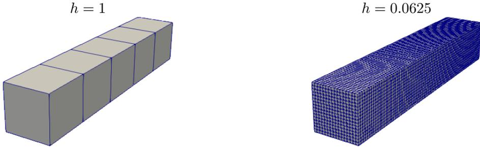
Figure 3.37: Example 2 - 3D cantilever beam: coarsest mesh for  $h = 1$  (left), refined mesh with  $h = 0.0625$  and four refinement steps (right).
