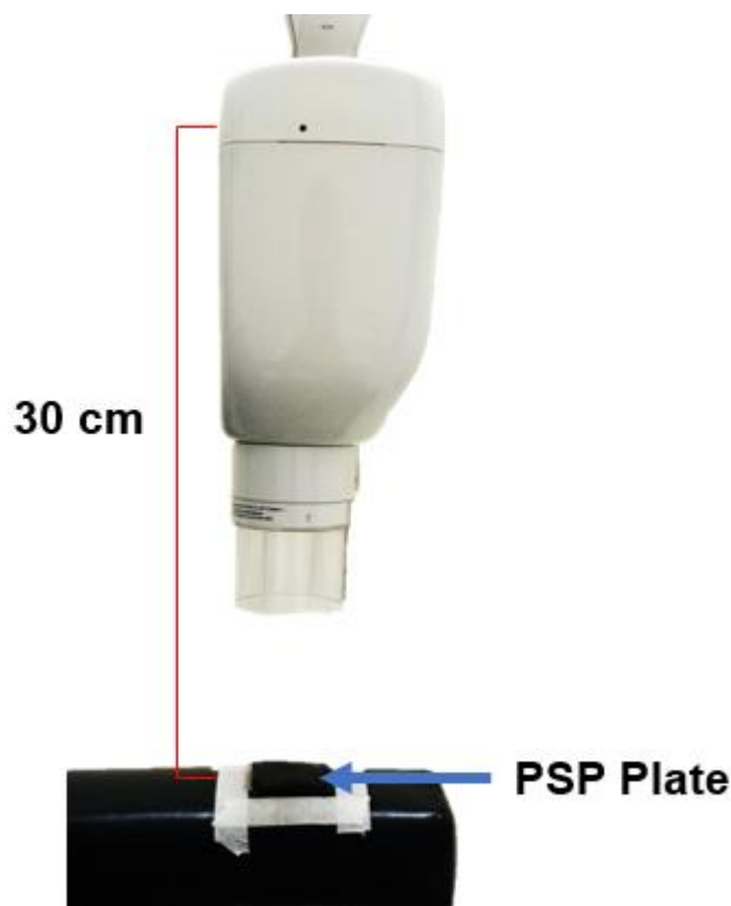
Figure 4. X-ray exposure setup with a focus-receptor distance of 30 cm.
