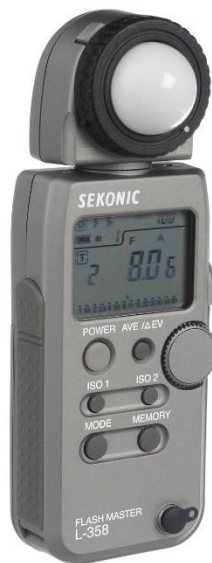
Figure 6. Sekonic L-358 photometer used to obtain the lamp illuminance.
