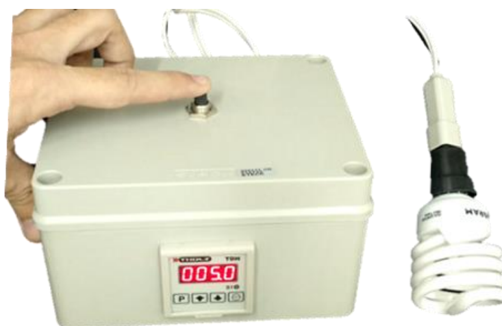
Figure 5. Custom-made device for controlled light exposure.
