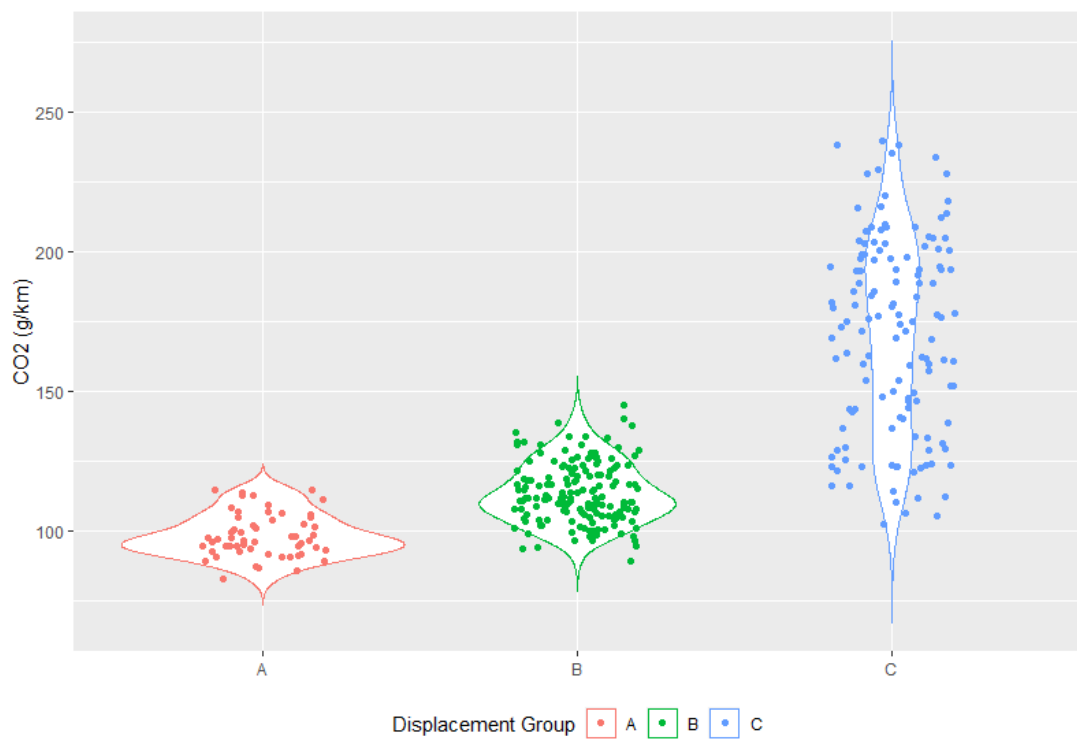
Figure 5.27: Fossil CO 2 emissions rates for displacement group. A refers to 1.0 liter engines, B for above 1.0l and below 2.0l, C for more than 2.0l. Values for 2021 from Inmetro (2022)
