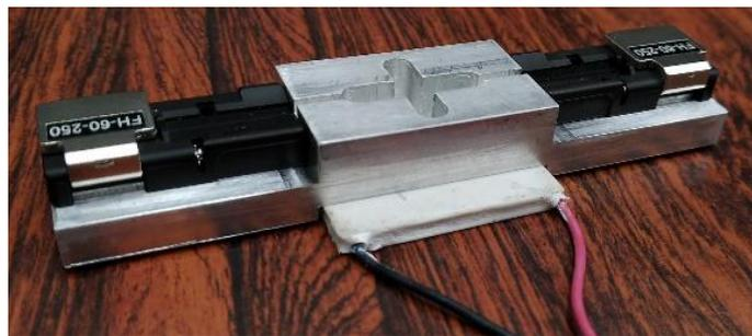
Figure 32 – Up: 3D model of the fiber bathing apparatus indicating its main features, such as alignment rails and a slot for a Peltier device. Down: Machined bathing apparatus with fiber holders and a Peltier device.
