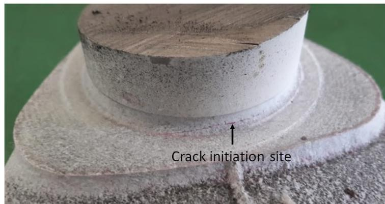
Figure 5.5 – Crack on the fillet radius surface of the original crankshaft model.
