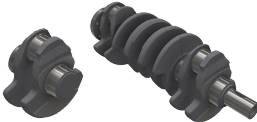
Figure 2.2 – Original crankthrow and crankshaft geometry.
