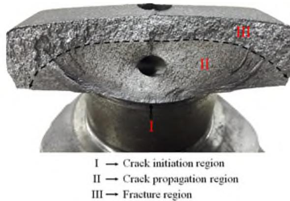
Figure 5.8 – Crack propagation regions in the crankweb of the lightweight crankshaft model.
