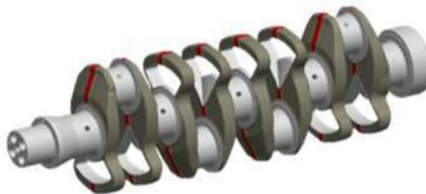
Figure 2.16 – 3D model geometry of the crankshaft modified by Rodrigues (2013).
