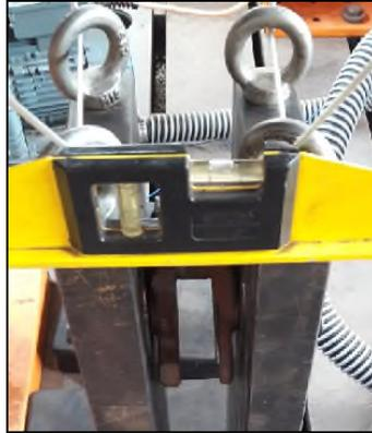
Figure 4.13 – Spirit level used in the bending test rig alignment.
