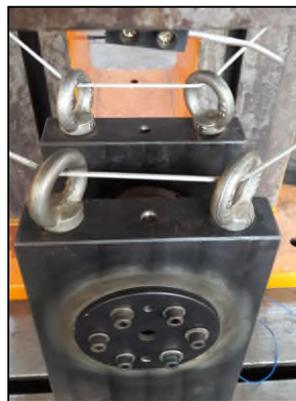
Figure 4.12 – Bending test rig suspended by wires through the lifting eyes.
