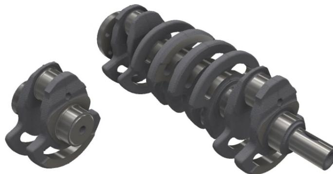
Figure 2.12 – 3D geometries of the lightweight crankthrow and crankshaft.
