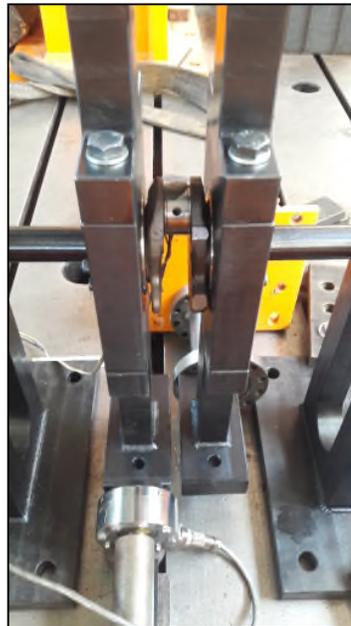
Figure 4.3 – Setup of the torsion static calibration.
