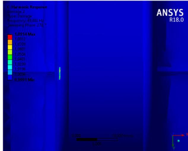
Figure 5.13 – Damage in the fillet radii of the original crankshaft for acceleration of 6.43 g.
