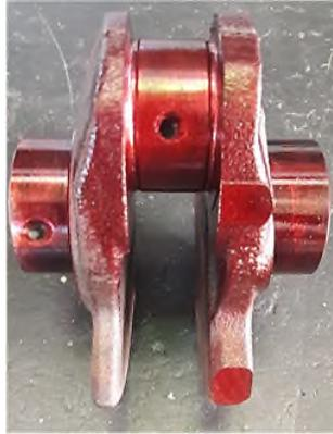
Figure 5.4 – Penetrant liquid applied to the crankshaft specimen.
