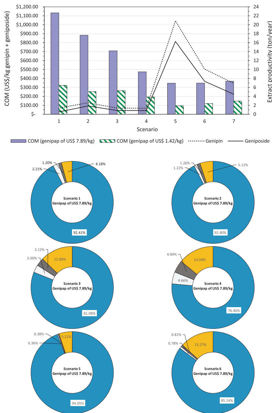
Fig. 7. Cost of manufacturing, extract productivity, and the main percentual contribution costs on the total cost of manufacturing of genipap pulp at industrial-scale with ethanol recycle.
