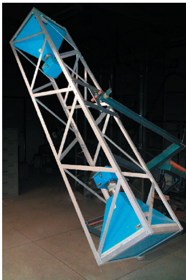
Fig. 1. One of the five Tupi telescopes; each one is constituted by two detectors (plastic scintillator 50 cm \times 50 cm \times 3 cm) within the pyramidal box at the top and bottom positions. On top of each pyramidal box is a (3-inch) photomultiplier. The separation between the detectors is 3 m. (Color online)
