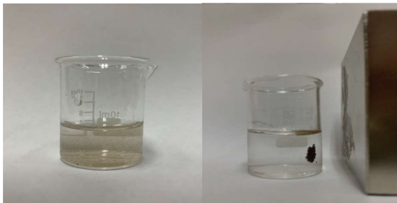
Figure 3.7 – GO/mCS/OC separation with magnet.
