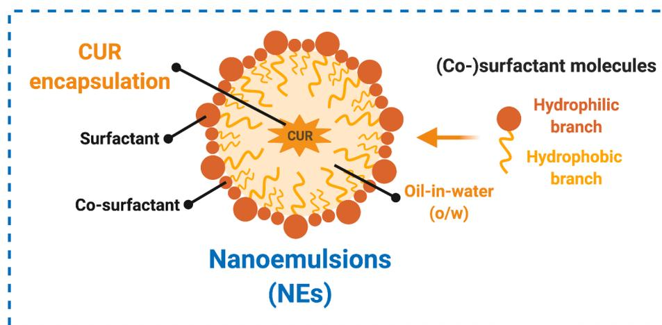
**Fig. 5.** Schematic representation of oil-in-water (o/w) nanoemulsion (NEs) loaded with a hydrophobic drug, curcumin (CUR). NEs are formed by nano-scale droplets that contain an oil phase in the core dispersed in bulk aqueous phase (or vice-versa – w/o), with the help of an interfacially active compound (*i.e.*, surfactant). Based on Yoon et al. (2018) and Pachioni-Vasconcelos et al. (2016).
