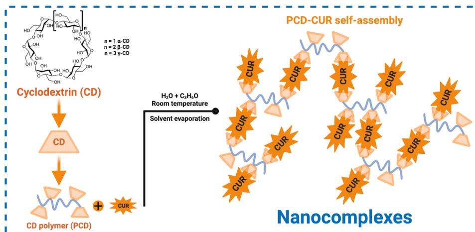
**Fig. 7.** Schematic representation of polymeric  $\beta$ -cyclodextrin/curcumin (PCD/CUR) self-assembly through the inclusion complexation mechanism formation, based on Yallapu et al. (2010).
