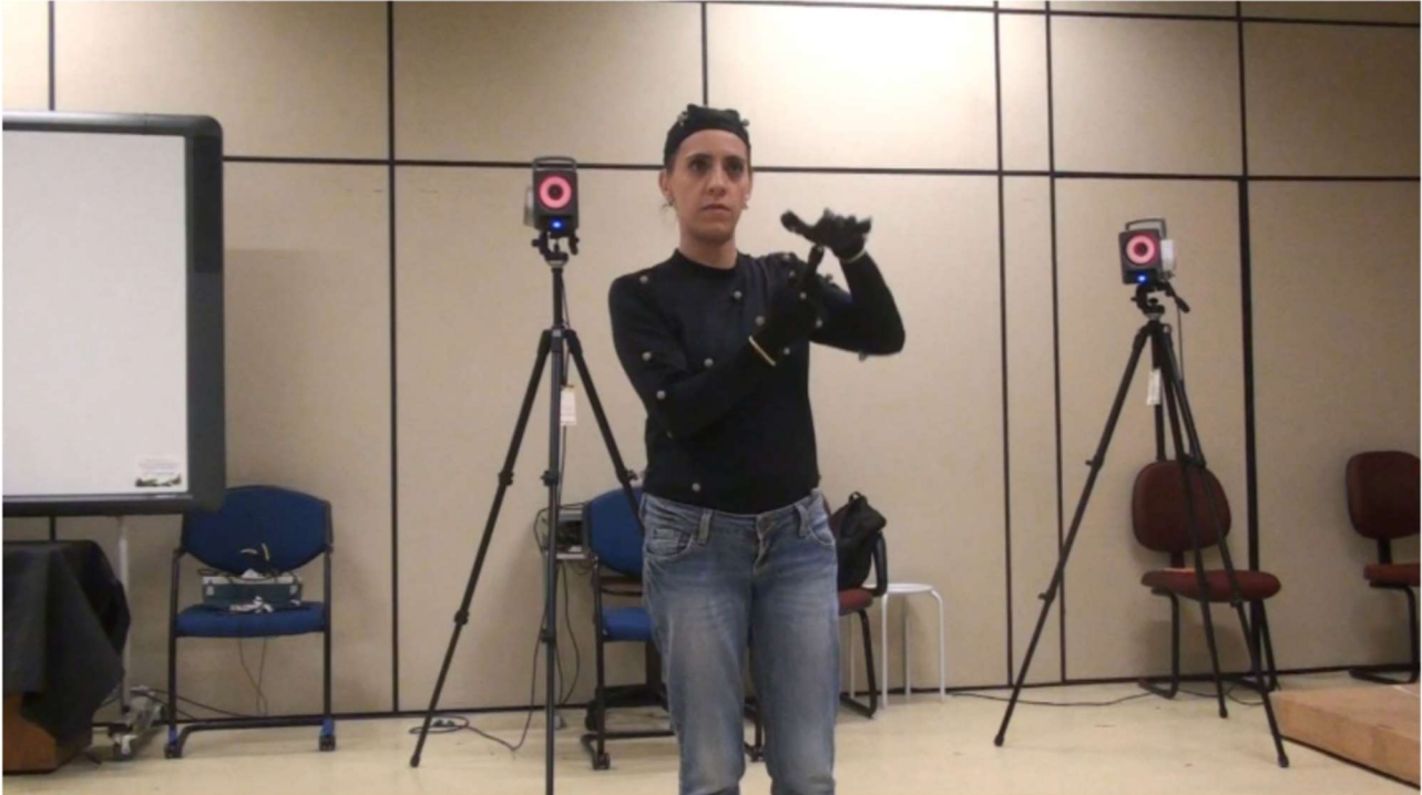
Figure 3. 2. Motion capture session at CTI facility. 2 infrared cameras can be seen on both sides of the interpreter, who is wearing the standard black clothes with the reflective markers (grey spheres).
