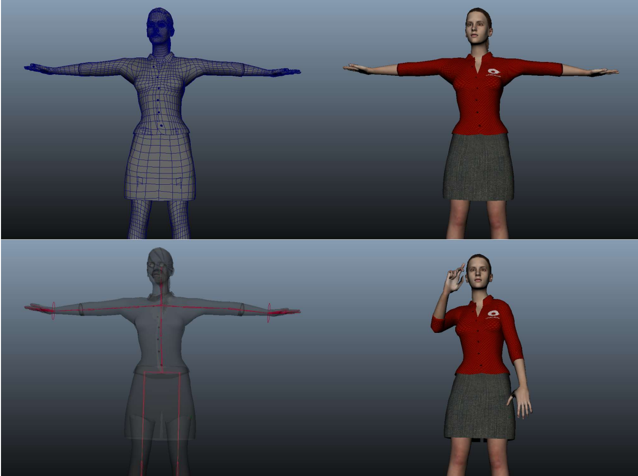
Figure D. 6. Examples of different sub-stages of a 3D animation production stage - modeled mesh (top left) with polygon edges in blue; textured model (top right); rigged character (bottom left) with the skeleton joints shown inside the polygonal mesh and the hands' controls as circles on the wrists; and animated/posed/signaling character (bottom right). Model derived from MAKEHUMAN (2016).
