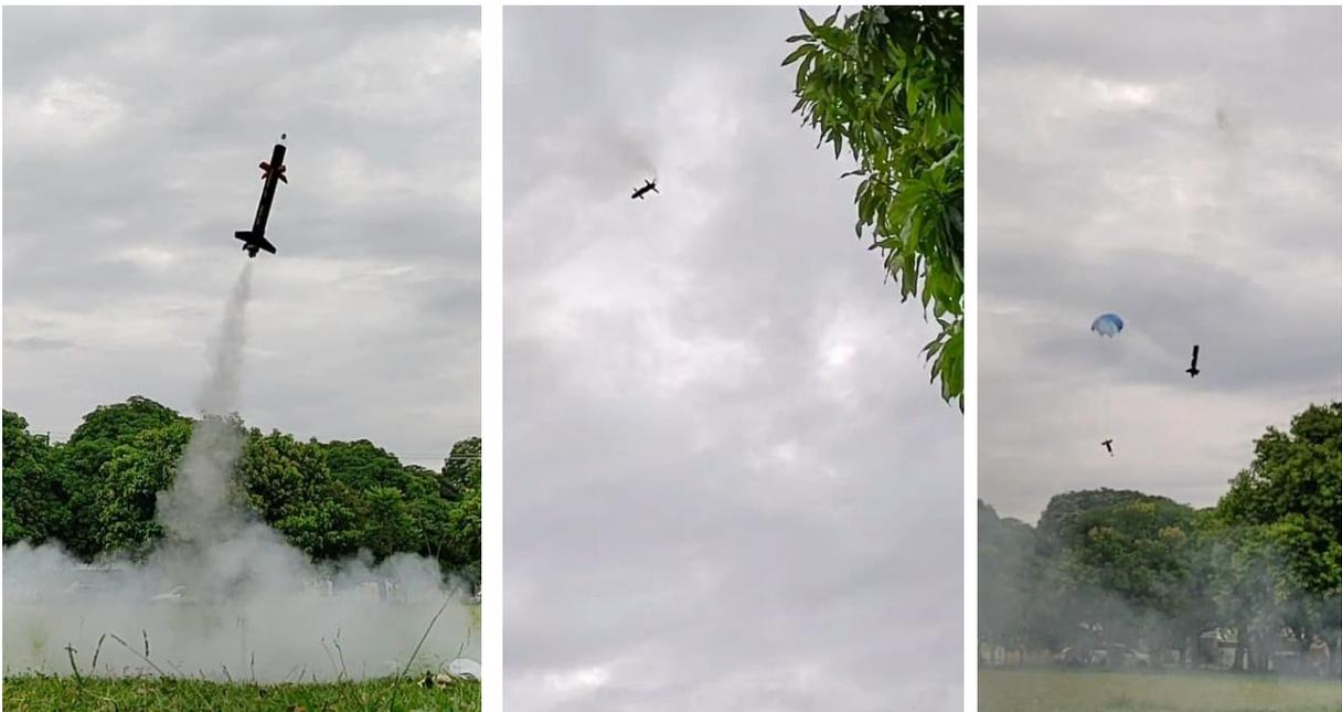
Figure 33. Rocket launch test without the onboard electronics.
