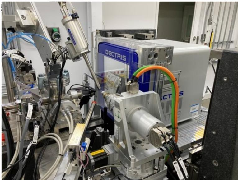
Figure 4.5: Current status of MicroManacá facility: Pilatus 2M (Dectris) detector, cryojet, on-axis video microscope, airbearing goniometer, beam stopper, slits and beam positioning monitors (BPM).
