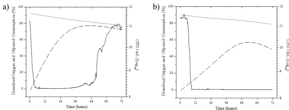
**Figure 4.** Fermentation parameters – AGG (a); CGBP (b) - microbial growth (-----), dissolved oxygen (—) and glycerol consumption (·····).
