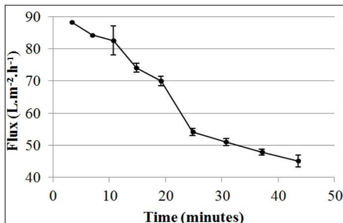
**Figure 4.** Flux of ultrafiltration (—).
