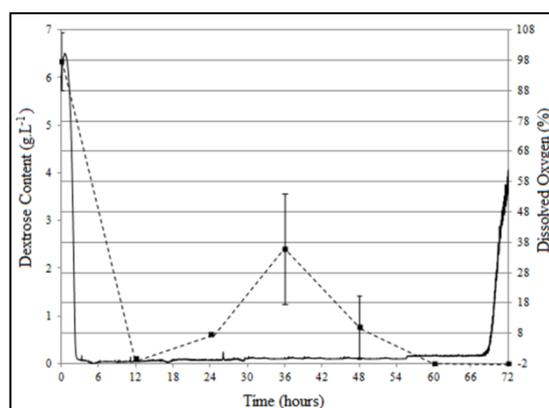
**Figure 3.** Dissolved Oxygen, (—), Dextrose Content (—■) during the fermentation of *Bacillus subtilis* LB 5a and production of surfactin.
