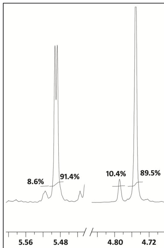
**Figura 8.** <sup>1</sup>H NMR data in CDCl<sub>3</sub> of purified sample and the presence of a second stereoisomer between 8% and 10%, which was based on signals of protons H-2 (5.49 ppm) and H-1 (4.76 ppm).
