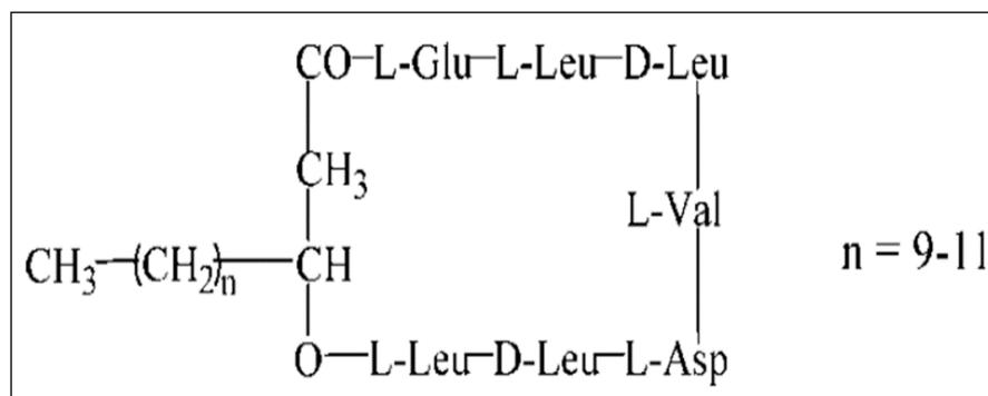
**Figure 1.** The chemical structure of surfactin [21].
