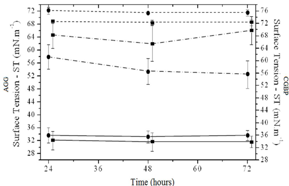
**Figure 5.** The ST, CMD-1 and CMD-2 values for the centrifuged culture media; bench fermentation: (■) experiments with CGBP [(—■—) ST, (•-■-•) CMD-1, (•-■-•) CMD-2], - (●) experiments with AGG: [(—●—) ST, (•-●-•) CMD-1, (•-●-•) CMD-2].
