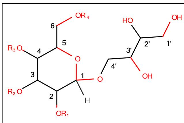
$\text{R}_1$  and  $\text{R}_2$ = Fatty acids;  $\text{R}_3$ = H;  $\text{R}_4$ =  $-\text{C}(\text{O})\text{CH}_3$
