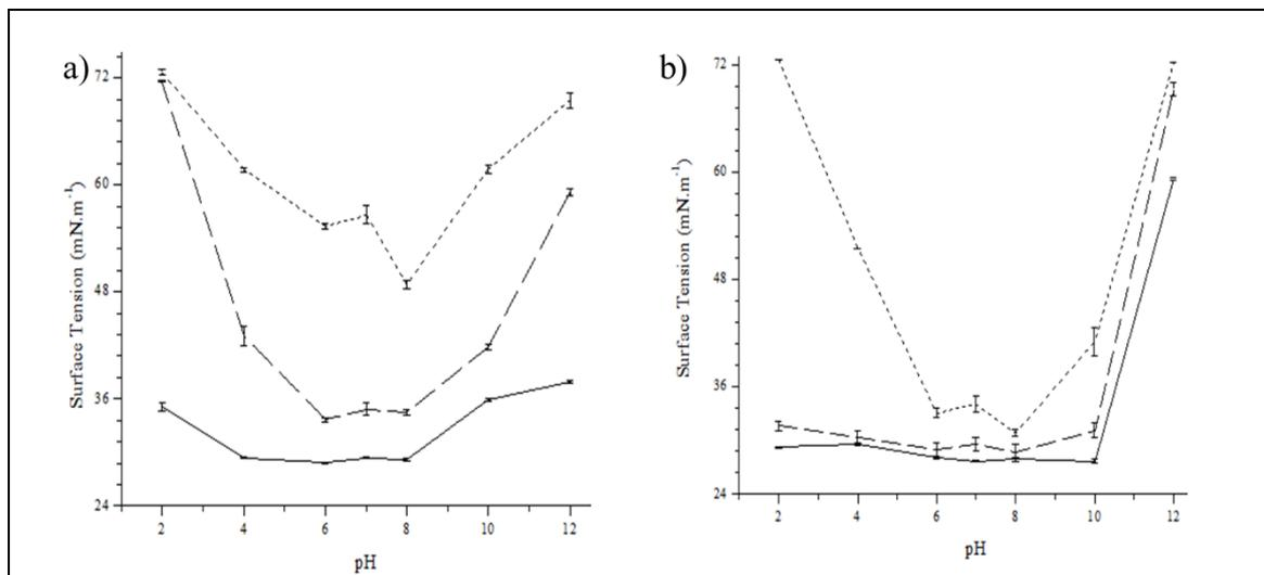
**Figure 3.** Surface activity of biosurfactants - surfactin (a) and MEL (b) - at range of pH; ST (—); CMD-1 (---); CMD-2 (.....).
