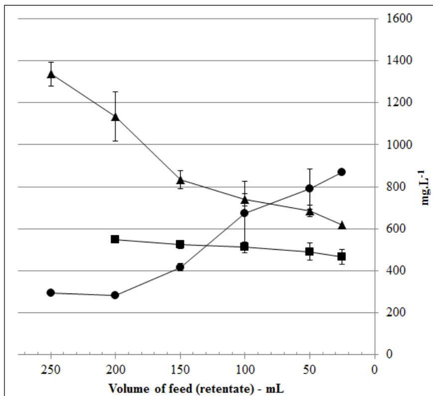
**Figure 5.** Concentration of MEL - feed/retentate (●), Concentration of protein - feed/retentate (▲); Concentration of protein - permeate (■).
