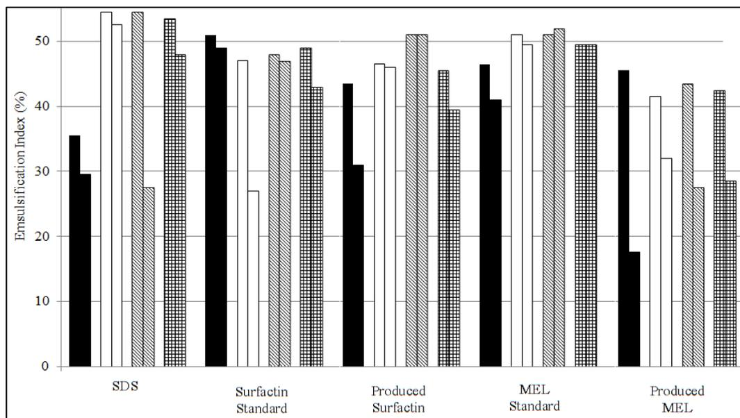
**Figure 8.** Emulsification Index of vegetable oils (%) – E<sub>24h</sub> (left) and E<sub>120h</sub> (right)
