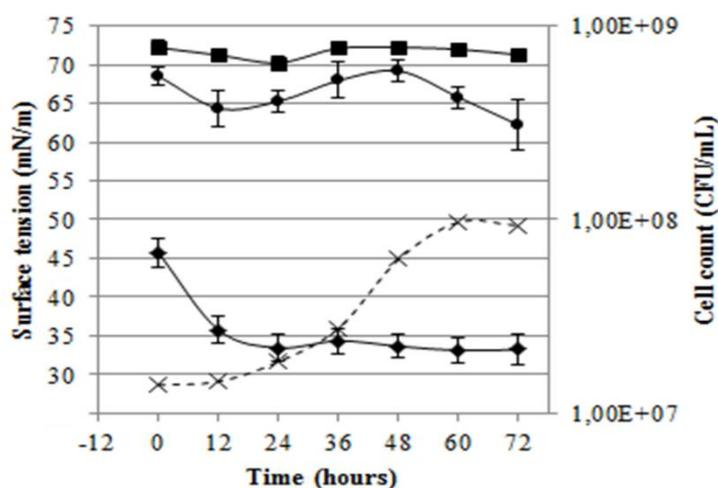
Figure 2. Growth curve and surface activity in the culture medium - raw glycerol from biodiesel industry plus peptone - (—◆—) ST; (—●—) CMD-1; (—■—) CMD-2; (---x---) Viable Cells.
