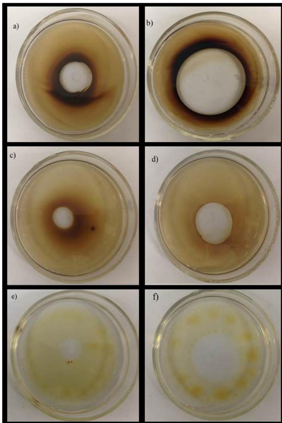
**Figure 6.** a) – Produced surfactin – heavy oil; b) produced MEL –heavy oil; c) Produced surfactin – medium oil; d) Produced MEL – medium oil; e) Produced surfactin – light oil; f) Produced MEL – light oil.
