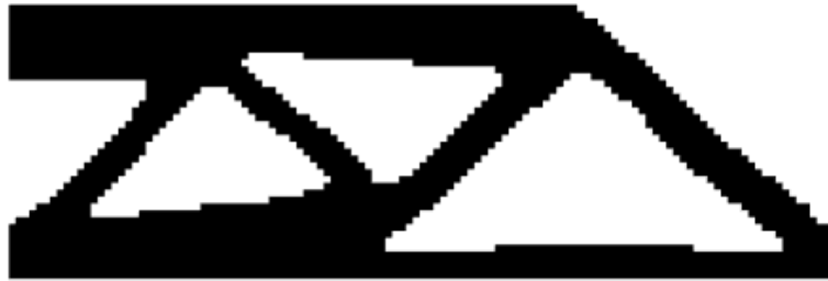
Figure 4.24: Final topology of the MBB beam obtained with BESO-FEM.
