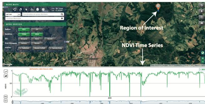
Fig. 1. Example of the NDVI time profile for a coordinate selected as a region of interest in satellite images.
