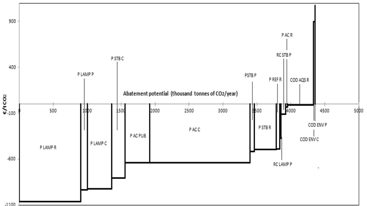
**Fig. 3** MACC for EE alternatives
