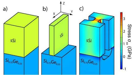
Fig. 1. Longitudinal stress ( $\sigma_{xx}$ ) simulation of (a) starting 30 nm thick strained Si grown on Si<sub>0.75</sub>Ge<sub>0.25</sub> SRB, (b) after conventional pattern of Fin structure and (c) after patterning and under etching of the Fins and contact pads. The full layer is in biaxial stress while the released Fin structure is under uniaxial stress.
