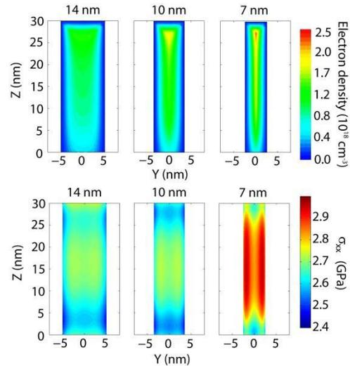
Fig. 3. (Top row) Cross sectional 2D simulations of charge density in trigate FinFETs using the 14, 10 and 7 nm nodes dimensions from Table I at gate voltage  $V_G = V_T$ . (bottom row) 2D longitudinal stress  $\sigma_{xx}$  simulations for Fins with the dimensions of the 14, 10 and 7 nm nodes.
