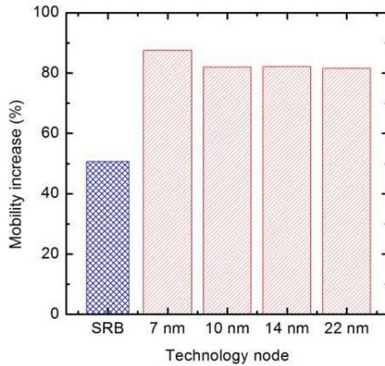
Fig. 4. Estimation of mobility increase in a n-type FinFET for different technology nodes using the patterning based strain technology (red). The mobility increase induced by SRB technology only is plotted for comparison.
